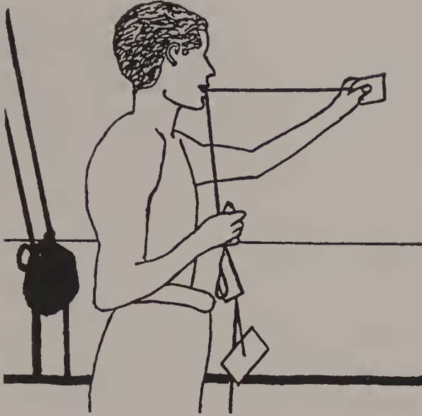
The kamal, a steering device consisting of a long, knotted cord with wooden squares at either end.
