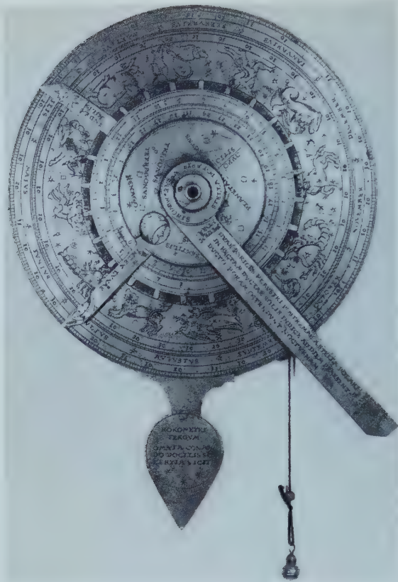
A brass nocturnal from Cologne, signed "Casper Vopeli' Faciele".
