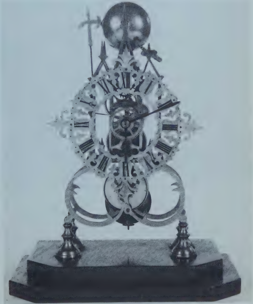
A typical mid-nineteenth century single-fusee skeleton clock with pierced chapter ring and passing strike of one blow at each hour. The power for running and striking comes from the single-coiled spring housed in the cylindrical case positioned in the lower centre area.
