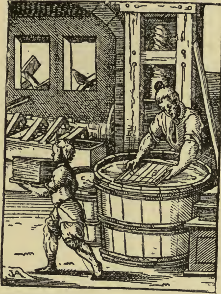
Fig. 147.—Workman engaged on the vat with the wire frame. Engraving by Jost Amman.
