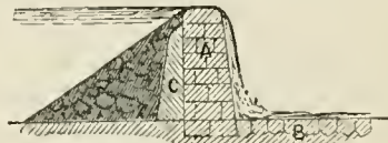
Fig. 5. A, masonry; B, pitching; C, clay puddle.
