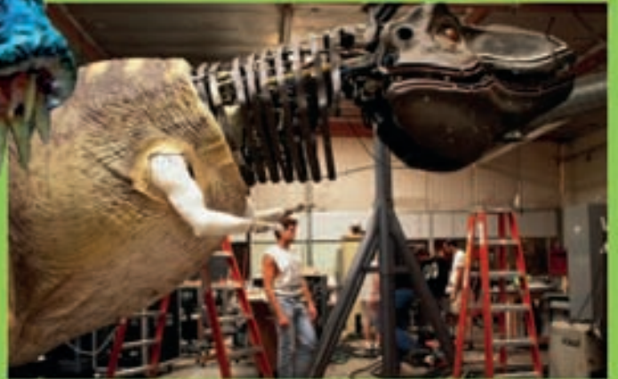
▲ A BIG COVER UP The dinosaur's skin is set over a plastic and steel frame, much of which has to be welded into position.
