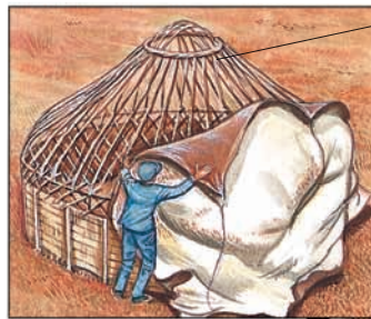
The framework of a yurt consists of a circular latticework frame with a central ring to support the roof. The frame is covered with felt lashed together with rope.
