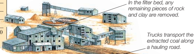
At the processing plant, the coal is cleaned and dried and sorted into different sizes.
