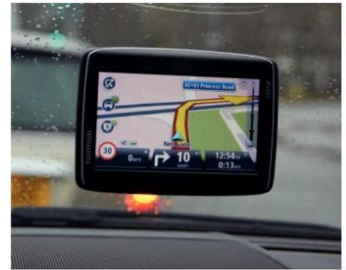
▲ Sat nav is a GPS receiver plus road maps. Type in the postcode for where you want to go, and it will show you the best route. The blue triangle here represents the car. Its position is continually updated.
