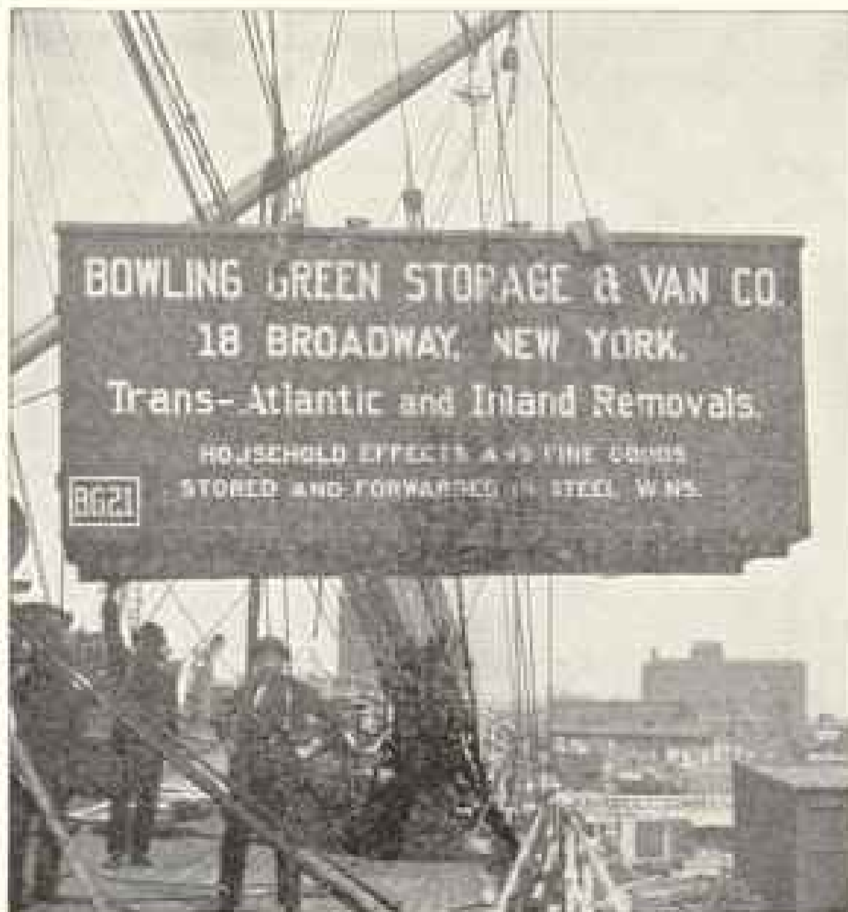
Hoisting Lift-van on Board Steamship
