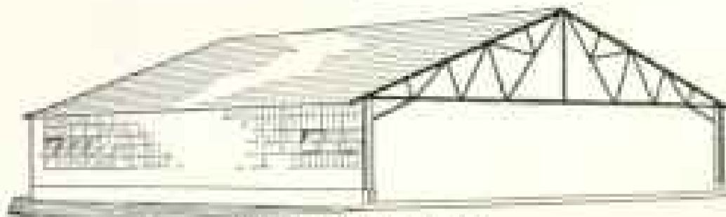
TYPE 1 (Clear Span) Widths—8'-12'-16'-20'-24'-28'-32'-40'-48'-50'-60'-68'
