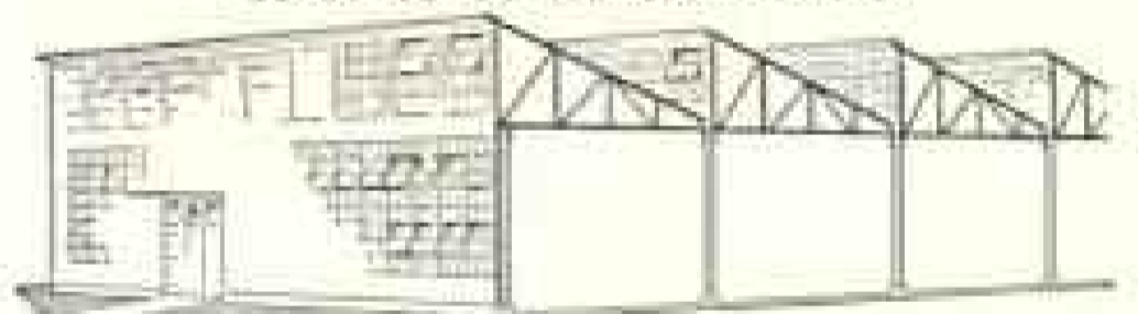
SAWTOOTH TYPE; Widths—Any Multiple of 28'-0"
