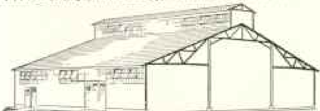
TYPE 3 (3 Bays) with Lantern; Widths—56'-60'-64'-68'-72'-76'-80'-84'-88'-96'-98'-100'-108'-116'
