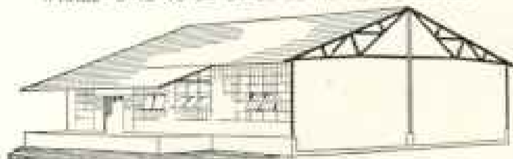
TYPE 2 (2 Bays) with Canopy; Widths—40'-48'-50'-56'-60'
