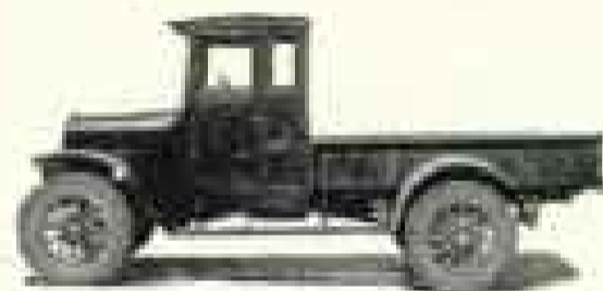
Model S International Speed Truck with open express body and enclosed cab. Three-quarter or semi-enclosed cab can be supplied.
