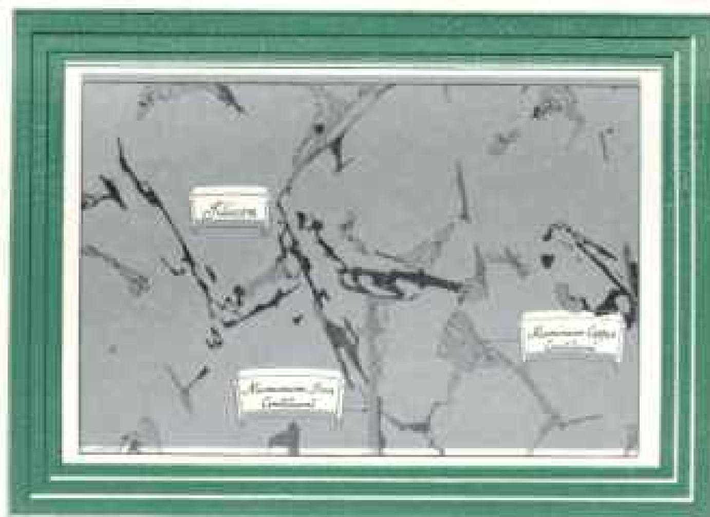
Photograph of a typical aluminum alloy, through a microscope to produce a magnification of 300 times.
