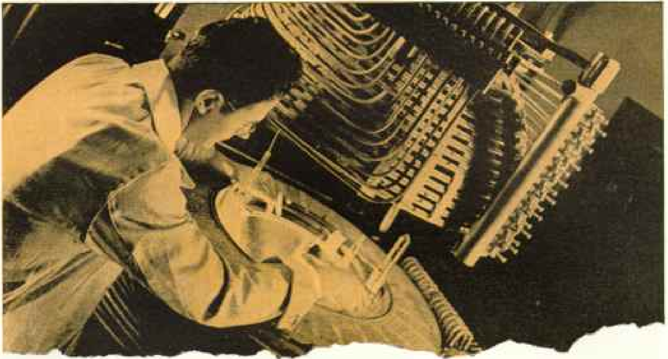
Helping the tire maker: Pictured here is a laboratory model of the new Westinghouse-developed "mass spectrometer," an adaptation of which analyzes gases with incredible swiftness and accuracy. Right now, one of the most important of its many uses is speeding up tremendously a step in the making of synthetic rubber.
