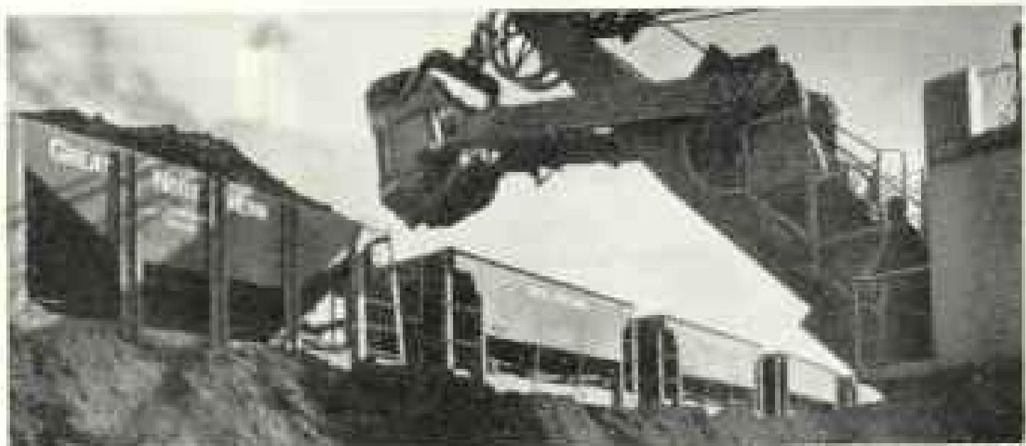
It requires only five "bites" of this giant power shovel to fill a 75-ton G.N. iron ore car.
