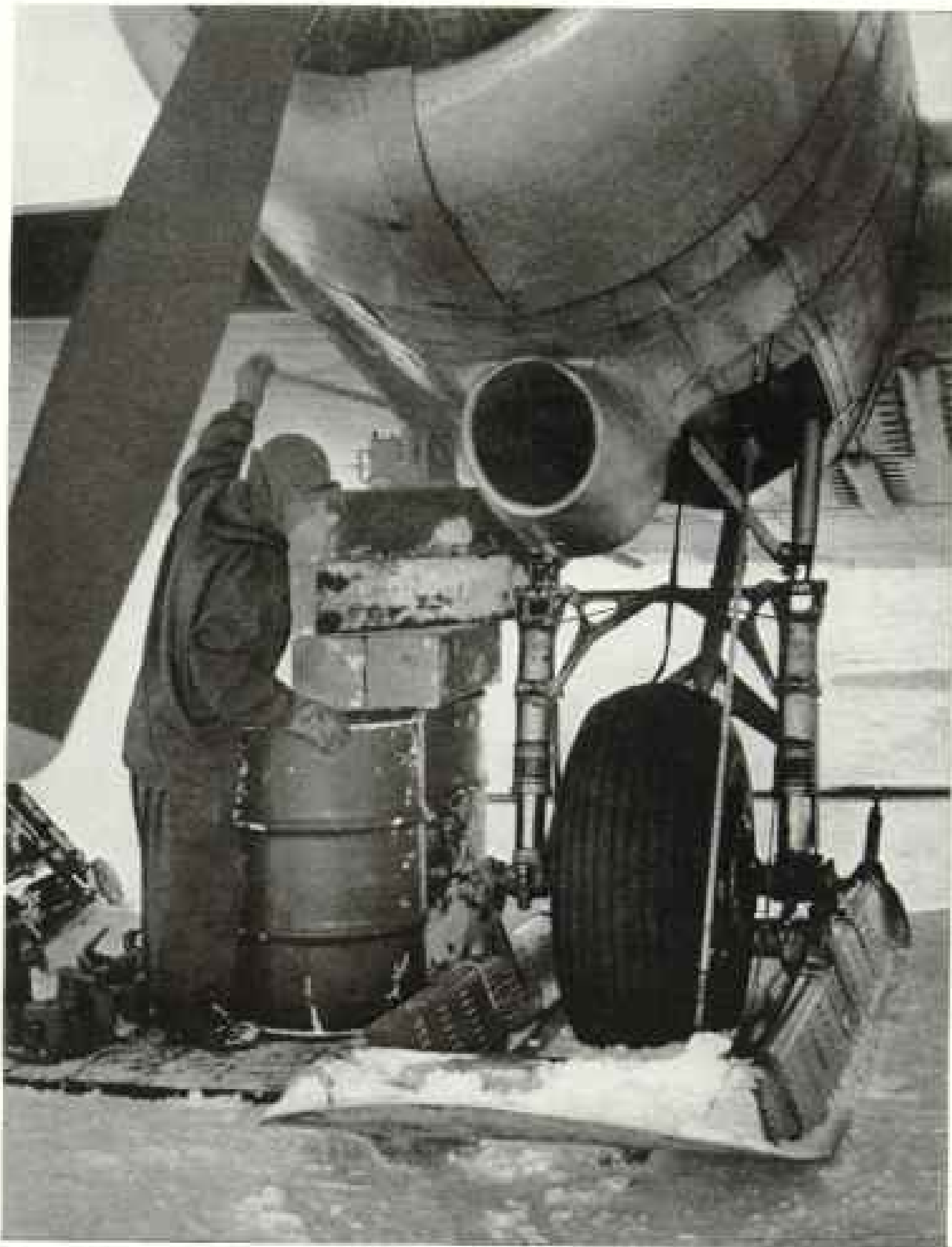
Ski-wheel Landing Gear Enabled the R4Ds to Take Off from a Carrier and Land on Snow
