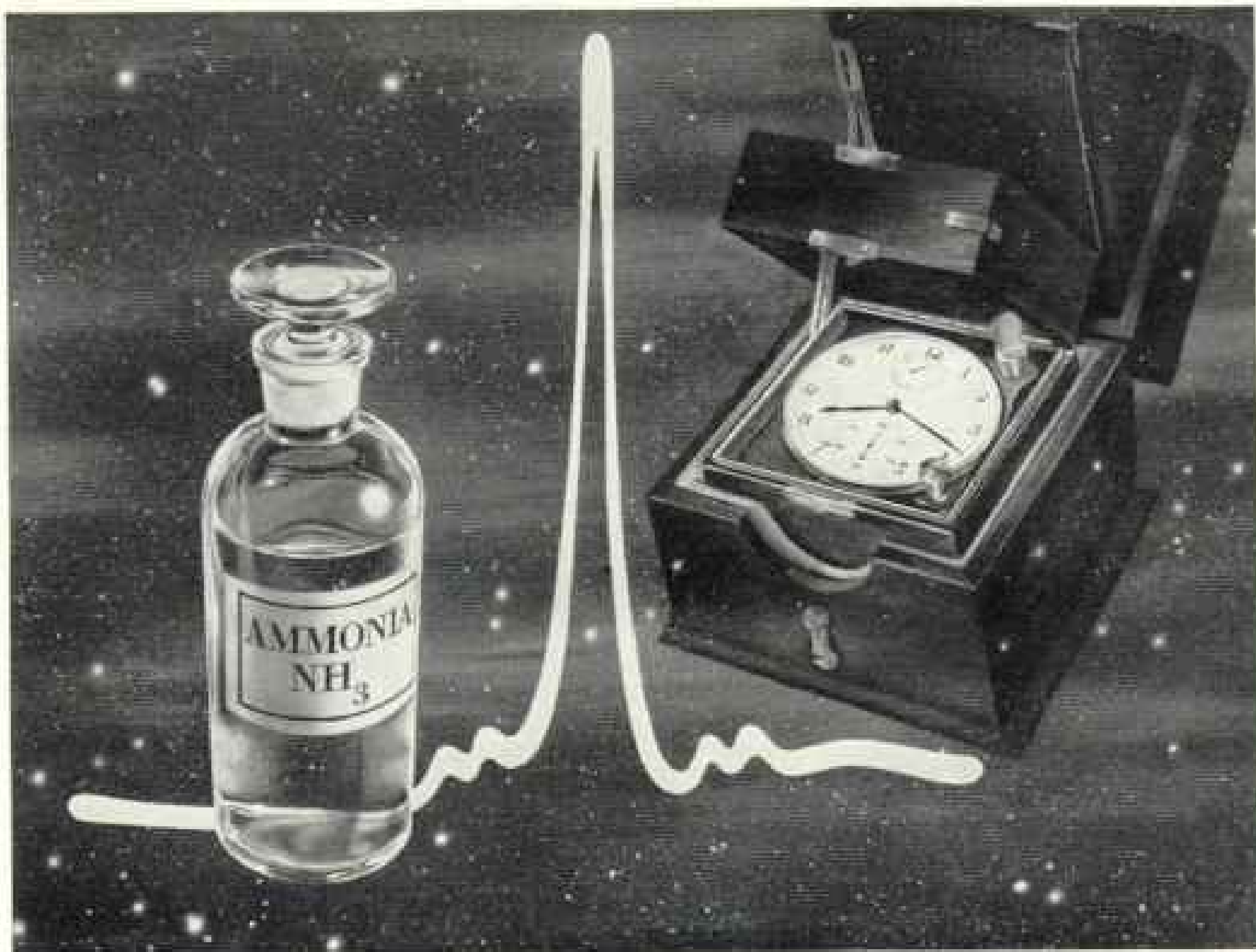
Using ammonia and radio waves, RCA scientists have devised a clock more accurate than the stars.
