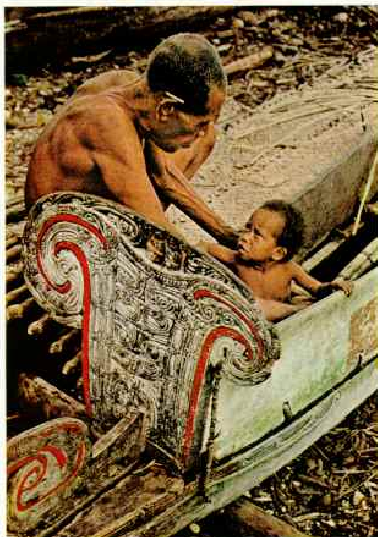
Craftsman hollows a log into a canoe. Upright ribs attached to the hull stand ready to receive the gunwales. Skilled sailors, Trobrianders still make ocean-going voyages in their dugouts.
