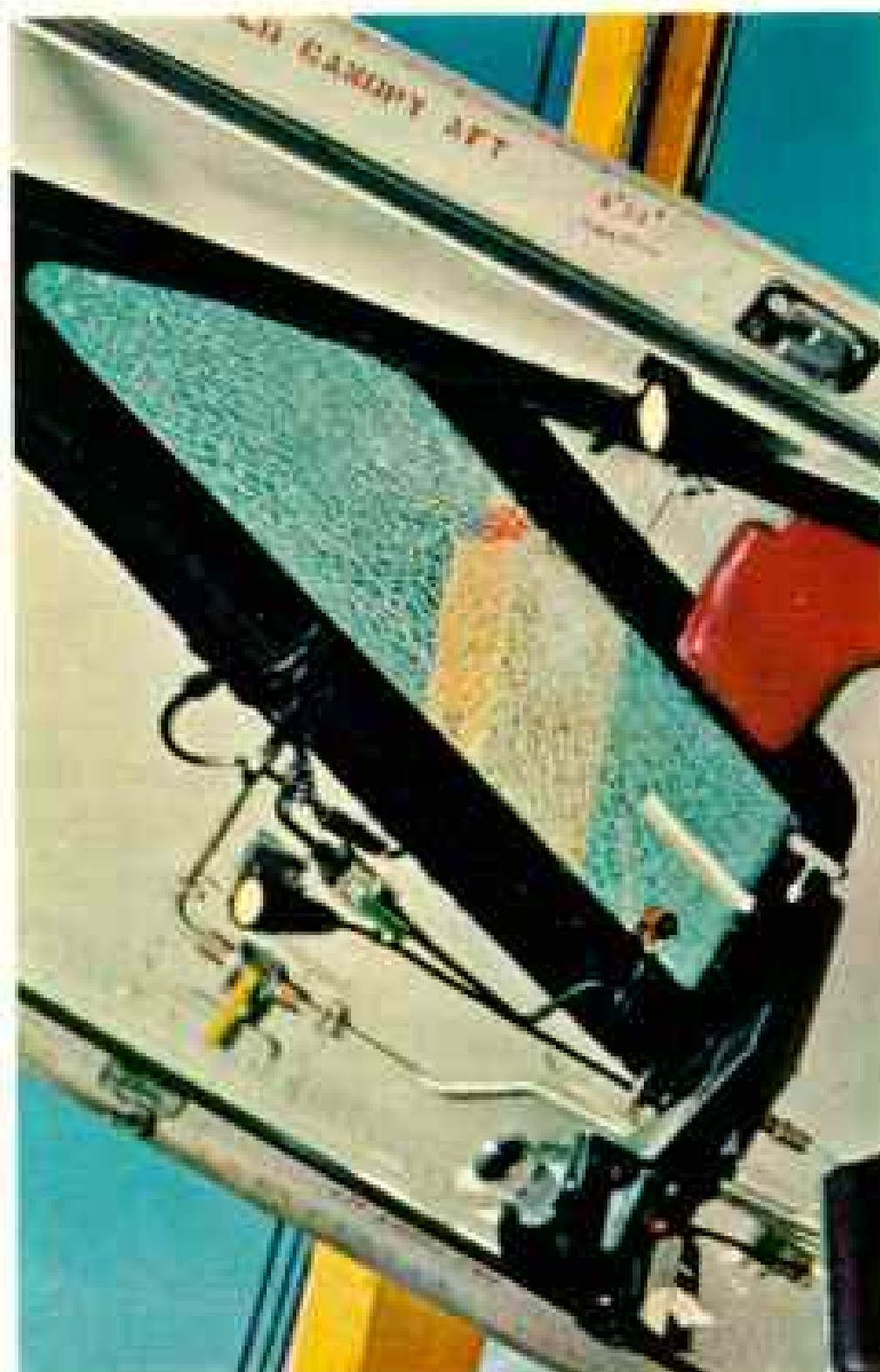
Right windshield cracked under the stress of hot metal, cutting Major White's vision in half.
