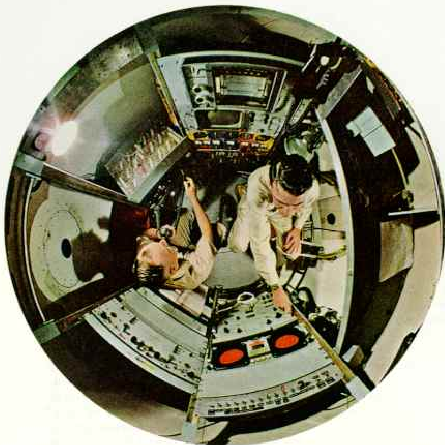
Cramped bathynauts sit hemmed in by batteries, echo sounder, gyroscope, TV, and controls. Lt. George W. Martin (left) telephones the surface; Commander Keach checks the sonar. Camera with 180-degree lens took the picture.
