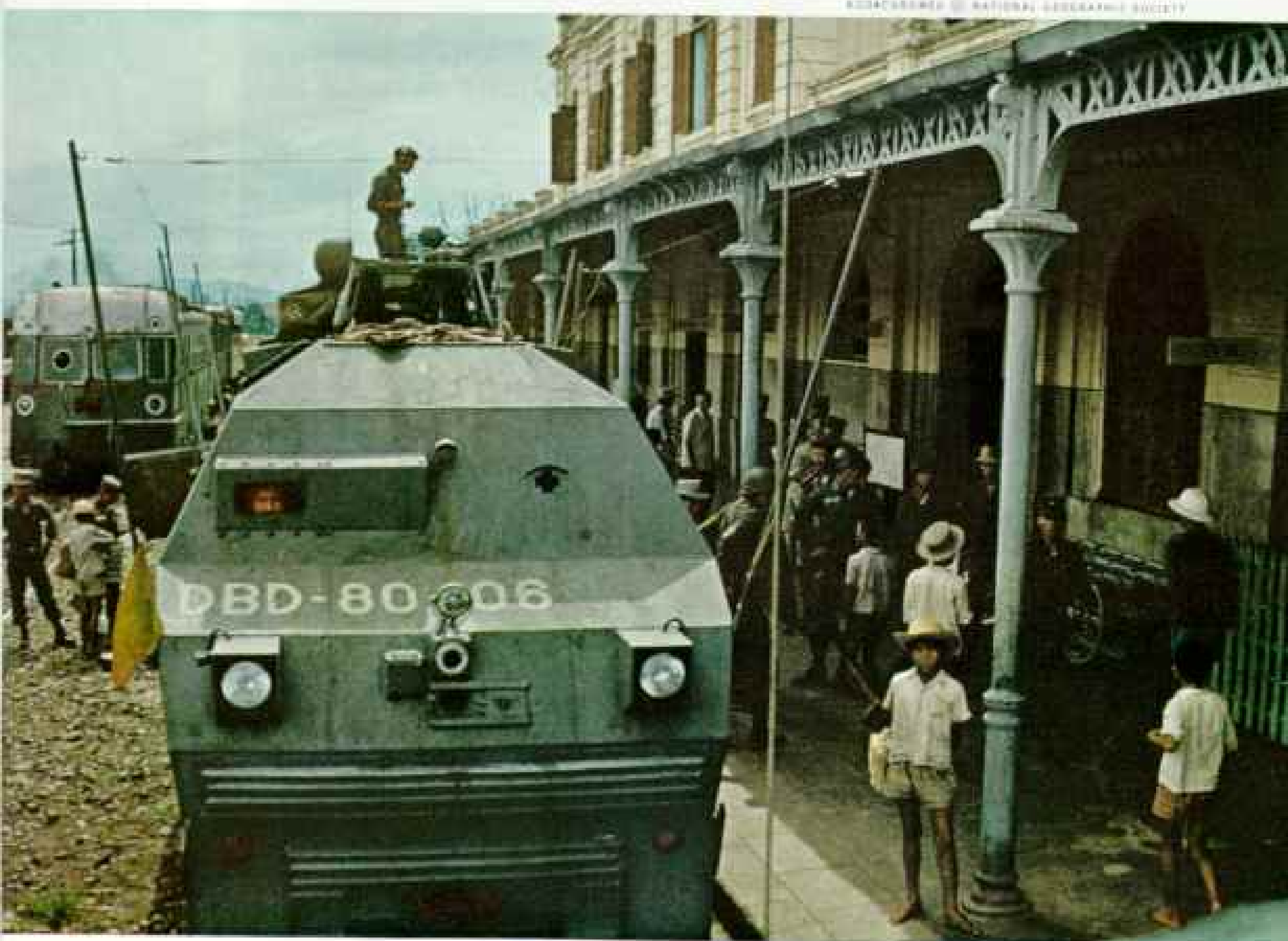
Sheath of steel with machine-gun turret protects a "Wickham trolley"—an armored car originally developed by the British during their war with Communists in Malaya. The author traveled in a service car (far left), normally reserved for railway inspectors.
