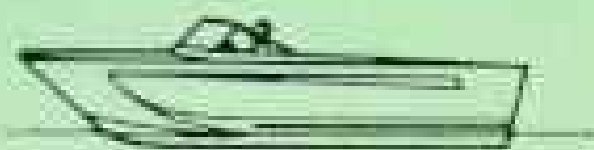
RUNNING—SIDE VIEW Bow stays low for excellent visibility. Sponsons stay just clear of surface.
