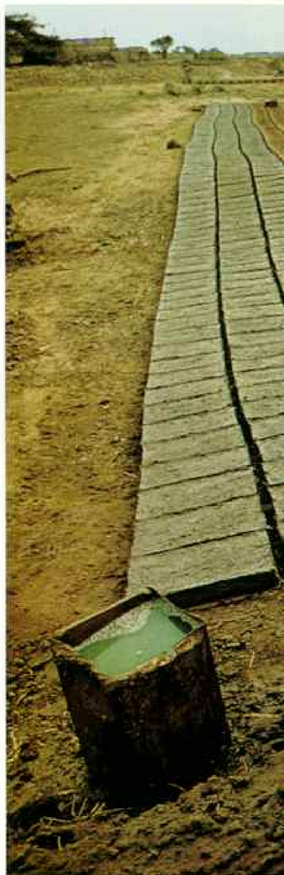
Building blocks for Trujillo houses, adobe bricks lie in ordered rows to dry; the brickmaker rinses his mold. Like his forebears of ancient times, he uses puddled mud—clay mixed with water—one of the few building materials the desert yields.
