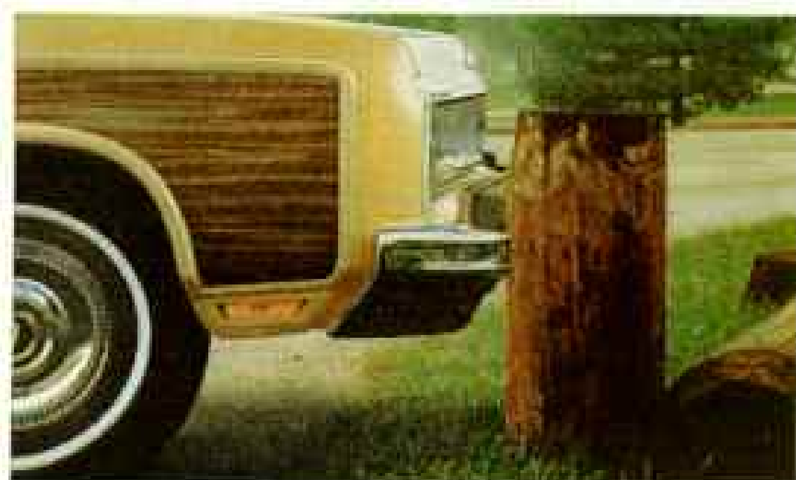
New improved front bumper system retracts on minor impact and hydraulically cushions the shock.
