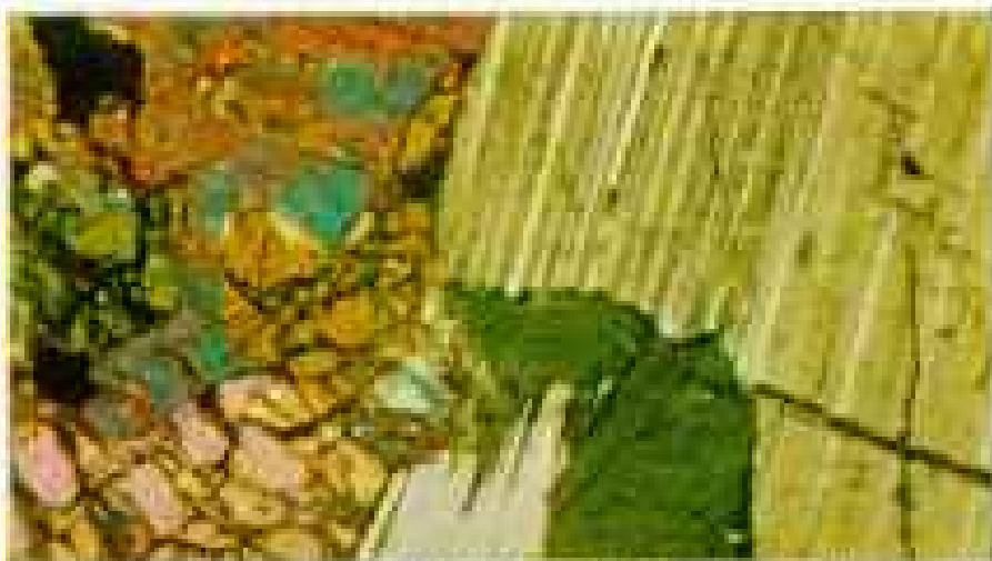
LAYER 3: GABBRO WITH CRYSTALS OF PLAGIOCLASE FELDSPAR (GRAY), PYROXENE (RED), AND OLIVINE (PINK), MAGNIFIED 45 TIMES
