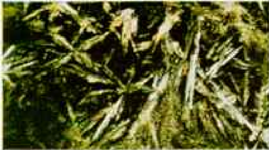
LAYER 2: FINE-GRAINED EXTRUSIVE BASALT WITH NEEDLES OF PLAGIOCLASE FELDSPAR, MAGNIFIED 40 TIMES
