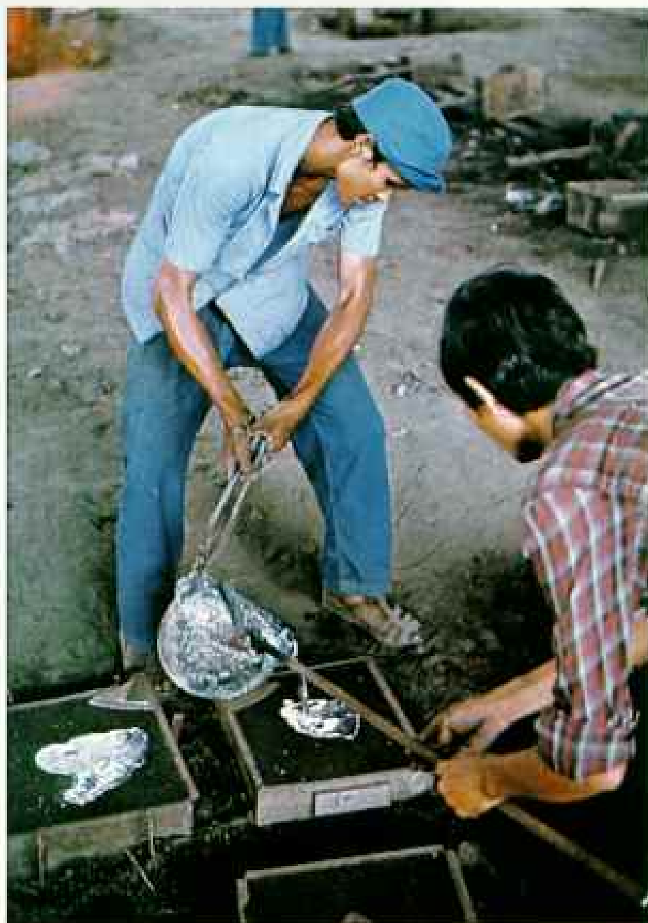
Doing peaceful duty in a Phnom Penh foundry, a U. S. Army helmet serves as a dipper for aluminum—from melted U. S. Air Force wing tanks—poured into molds to make cooking pots, which are in short supply. Under Pol Pot, the populace had to turn in their pots and pans and eat in communal kitchens.
