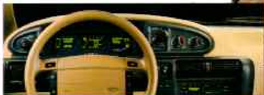
Ergonomically Designed Instrument Panel With Column-Mounted Shift.
