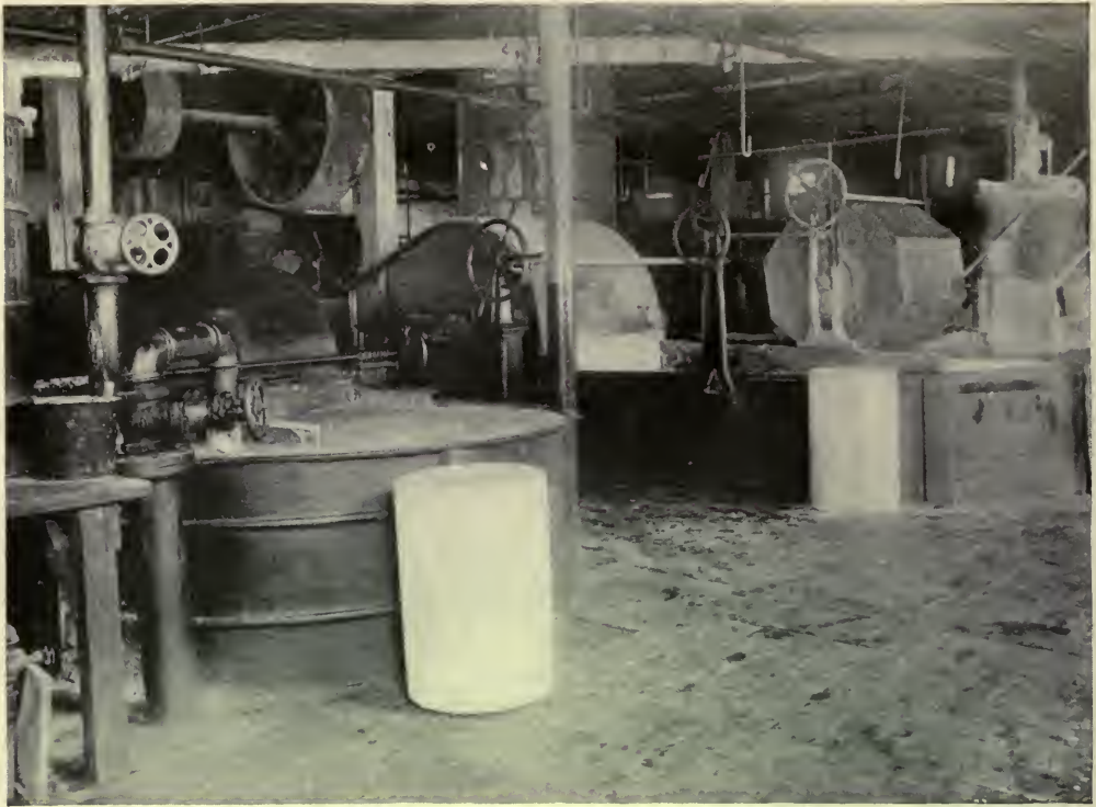
A CORNER OF THE BEATER-ROOM, WHERE THE DIGESTED WOOD IS FURTHER TREATED BEFORE BECOMING READY FOR CONVERSION INTO PAPER
