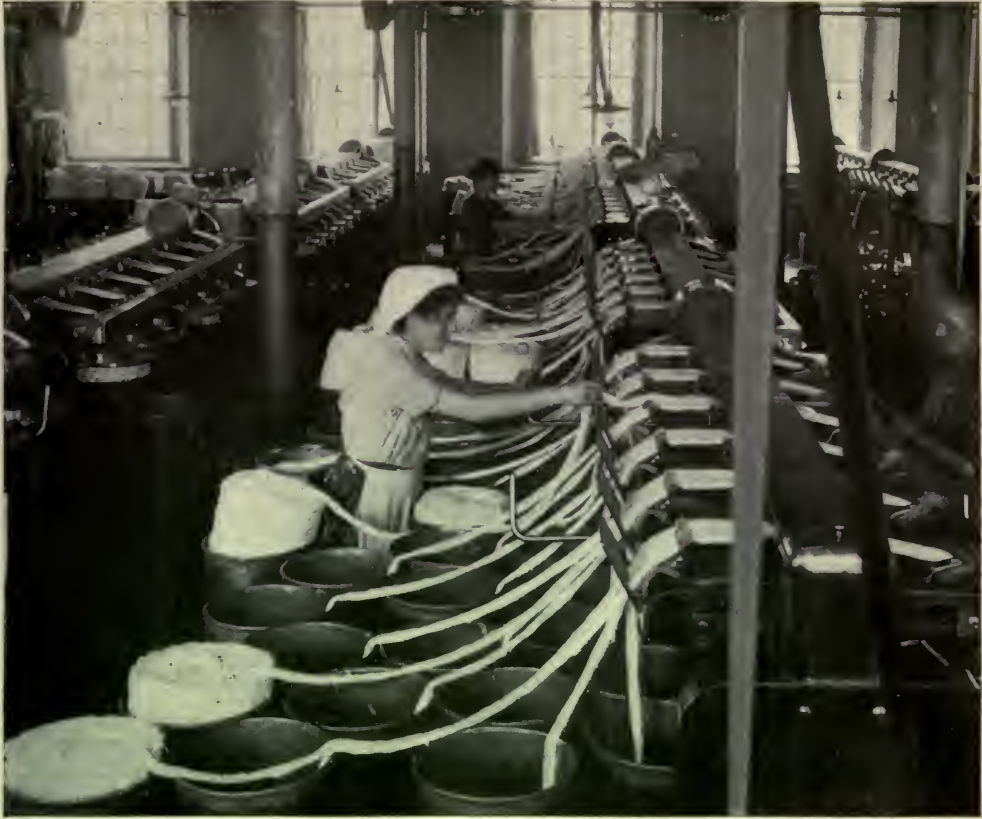
“DRAWING” SLIVERS IN A COTTON MILL, ONE OF THE STEPS PRELIMINARY TO SPINNING
