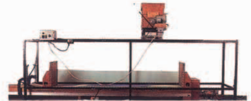
▲ MOUNTAIN MACHINE The paper and sand are held between fixed wooden blocks inside a tank.
