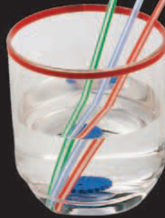
The break in the straws is an illusion caused by refraction.
