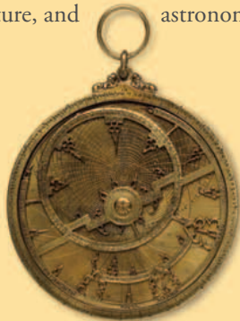
▲ ASTROLABE They perfected this instrument for calculating a person's position by using the Sun and stars.
