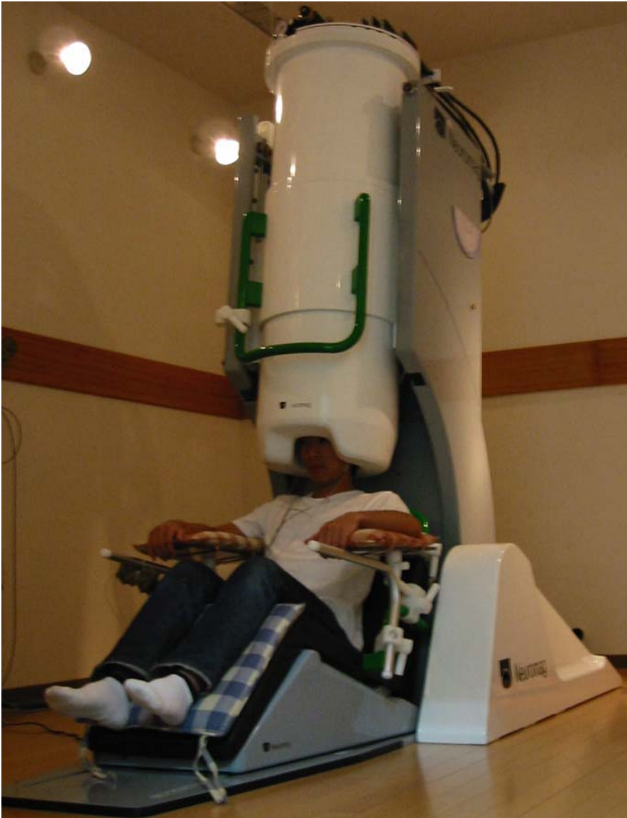
Photo 4.1 Magnetometer used in recording the MEG
