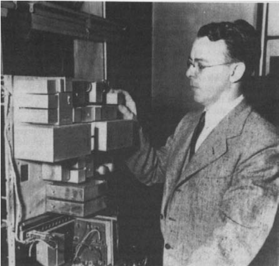
Figure 10.2 Black and a 1930 negative feedback repeater
