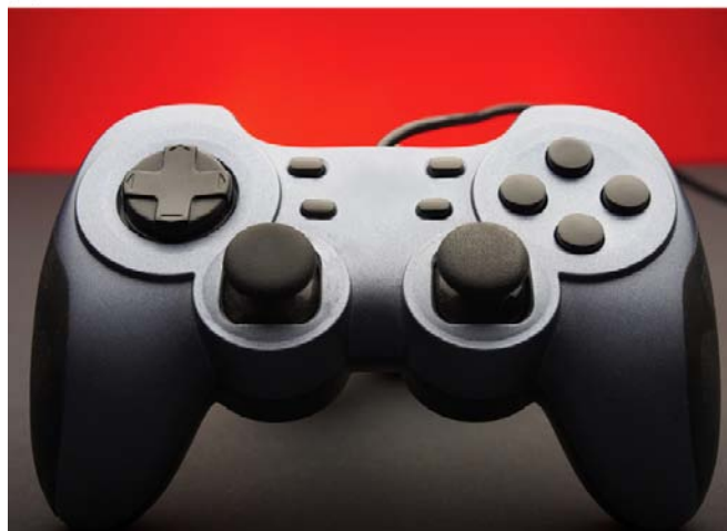
FIG. 11.10A & 11.10B Videogame controllers started out as a simple joystick and, as games became more sophisticated, progressed to a "gamepad" version. Photo courtesy iStockphoto. © kencameron, image #655730/orjp85, image #3845048.
