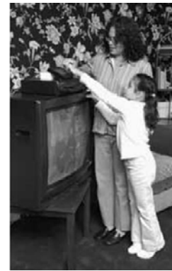
FIG. 8.4 The Nielsen people meter is attached to the viewer's television set. Courtesy Nielsen.
