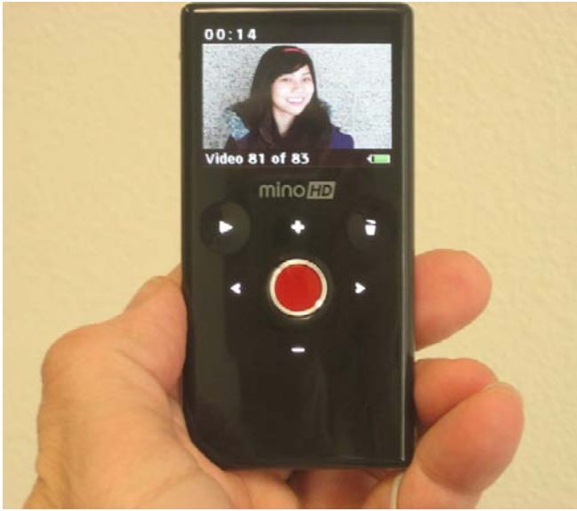
FIG. 10.5 This small camcorder records two hours of HD video and sound. Transfer of the video and audio to a computer for editing is done quickly and easily via a USB connector built in to the camcorder.
