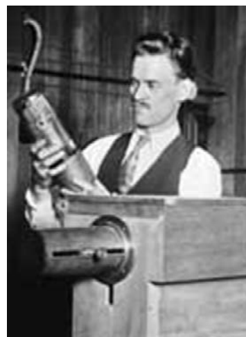
FIG. 3.3 Philo T. Farnsworth with an early television pickup tube. Courtesy MZTV Museum.
