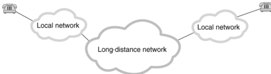
Figure 8.1 General structure of a PSTN.
