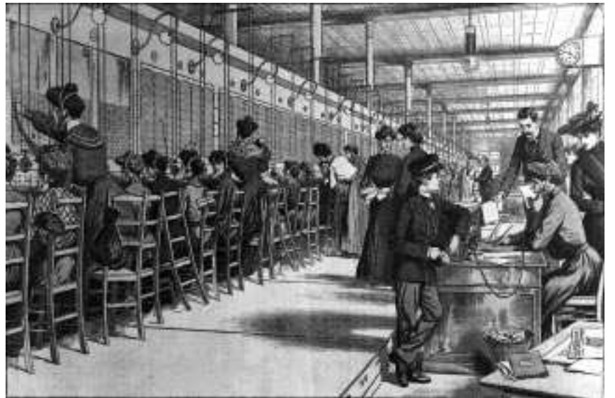
Fig. 5.7 Early telephone exchanges in Paris. (a) Operators work standing. (b) Operators are seated but still need to stand up for reaching the upper parts of the switchboard.
