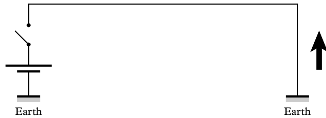
Fig. 4.2 One wire is sufficient! The Earth may take the place of the return wire.
