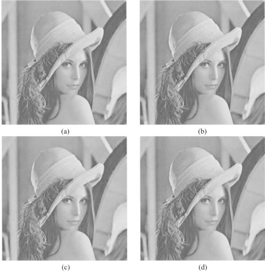
Figure 6.16. Reconstructed “Lena” when transmitted over noisy channels using the ERWIC algorithm (a) 0.25 bpp, BER=0.001 (33.10 dB). (b) 0.5 bpp, BER=0.001 (36.26 dB). (c) 0.25 bpp, BER=0.01 (32.19 dB). (d) 0.5 bpp, BER=0.01 (35.29 dB).
