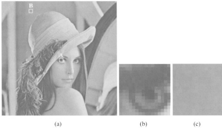
Figure 8.3. (a) Two different image-activity blocks. (b) Block A. (c) Block B.
