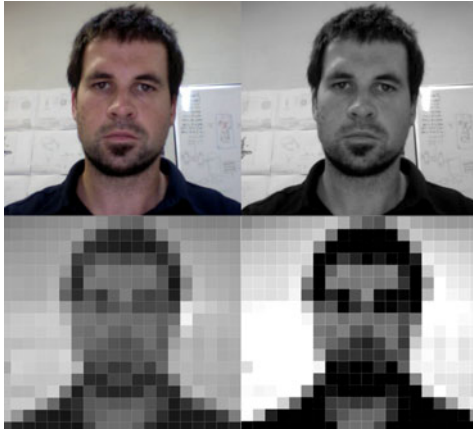
Fig. 10. Original image, greyscale conversion, pixel resize, covert to 4-bit
