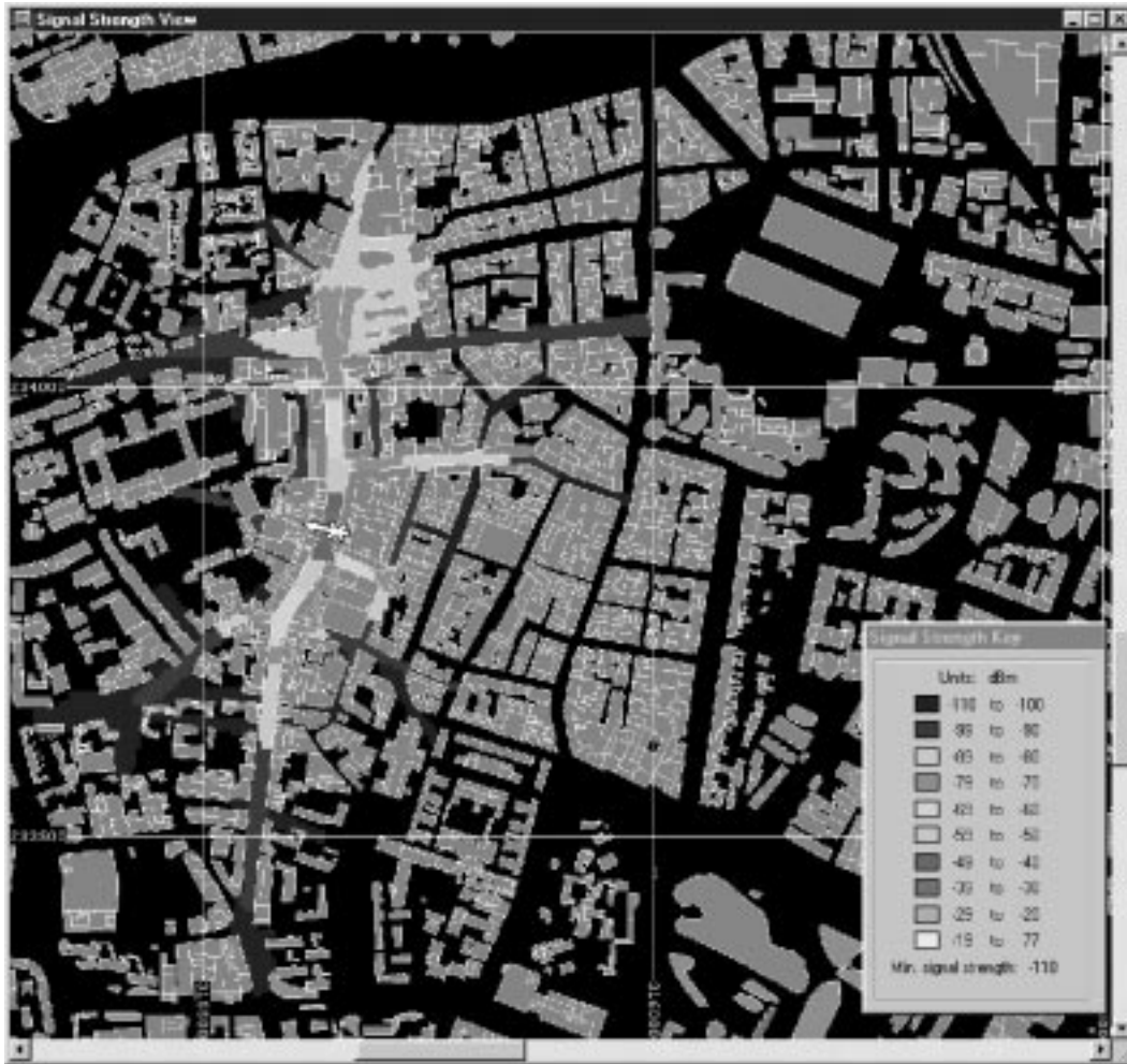
FIGURE 22.4: NP WorkPlace plot of a city street microcell. The map gridsize is 500 meters. The color version of this plot is presented elsewhere in this Handbook.
