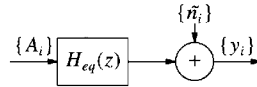
FIGURE 4.4: Equivalent discrete-time channel for the PAM system shown in Fig. 4.3 [ y_i = y(iT) , \tilde{n}_i = \tilde{n}(iT) ]
