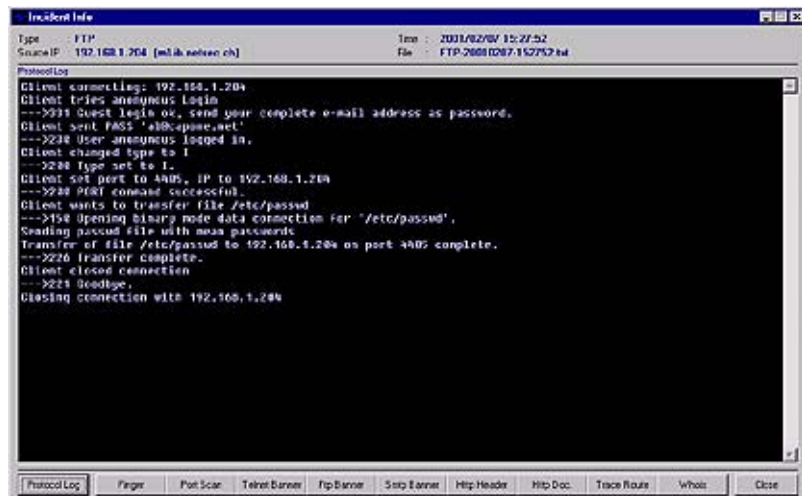
Figure 5.5 Log records from an attempt to download a UNIX /etc/passwd file
