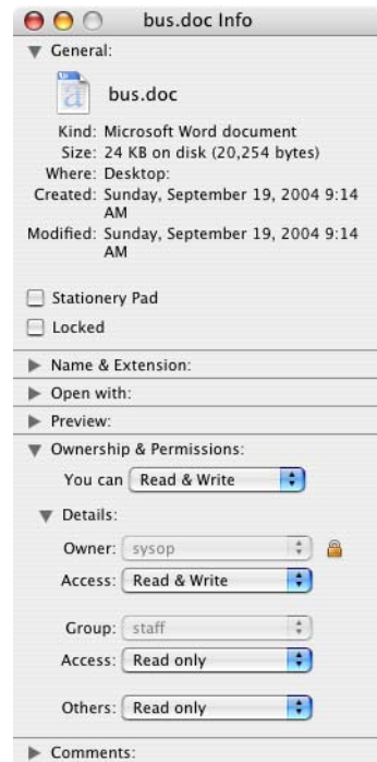
Figure 2.6 Using the Mac OS X GUI to change file or directory permissions
