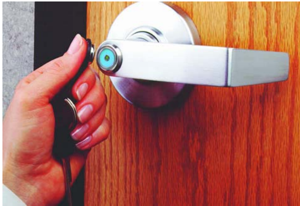
Figure 3.6 Using an iButton to unlock a door by placing the token against a sensor
