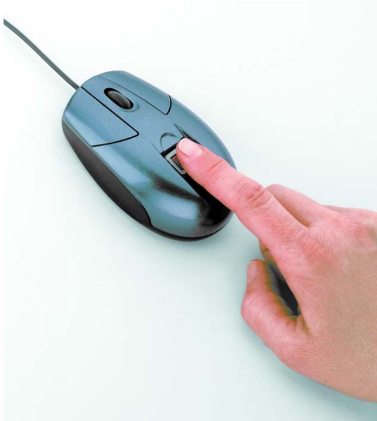
Figure 3.7 The Fellowes Secure Touch mouse with its fingerprint reader
