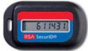
Figure 9.5 The RSA SecurID device that generates a one-time use password
