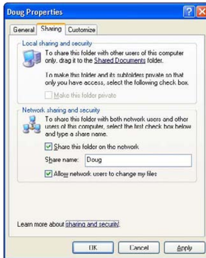
Figure 3-5: The Sharing options come to life when you select the Share This Folder on the Network check box (in Windows XP).
