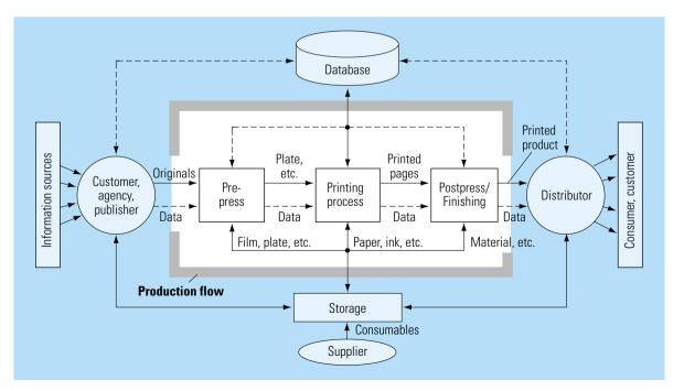
Fig. 1.2-1 Production flow, material and data flow for print media production
