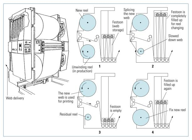
Fig. 2.1-81 Zero-speed web splicer (Buttler)
