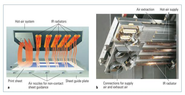
Fig. 2.1-58 Dryer module for the combination of IR radiation and hot air.
