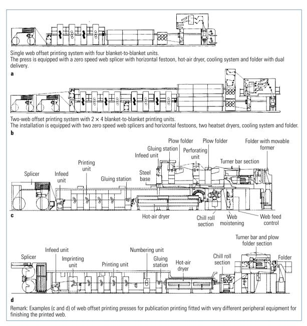
Fig. 2.1-188 Commercial web-fed offset printing systems ([2.1-7])
