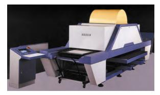
Fig. 3.1-23 Step-and-repeat machine (StarLight, Krause-Biagosch)
