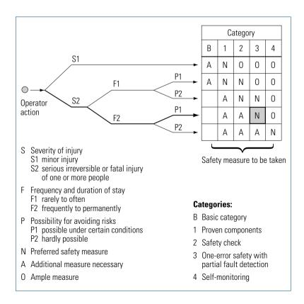
When using a computer or programmable controller as a *safety regulator*, safety-related malfunctioning must be detected and result in disconnection. Safetyrelevant control parts are, for example, emergency circuit breakers, electrical interlock circuits, and travel and speed limitations in inching mode.
