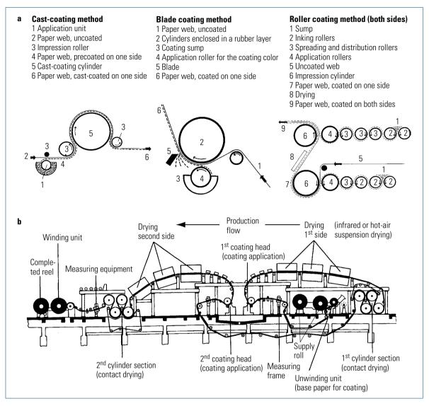
Fig. 1.5-6 Paper finishing by coating.
