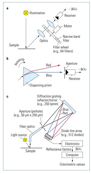
Spectrometer principles for measuring spectral reflectance factors. **a** Filter wheel principle:
