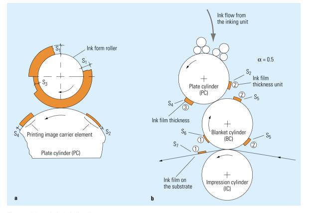
Fig. 2.1-8 Ink transfer in the inking unit.
