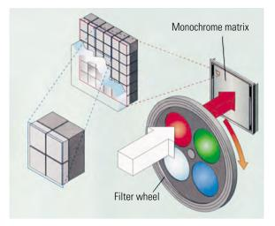
Color image recording with an area sensor; RGB color separation using three separate shots, each with alternating color filter via filter wheel; neutral filter for black and white shots (AGFA)
