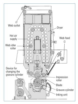
Fig. 1.3-16 Printing unit of a gravure printing press
