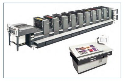
Speedmaster SM 74 with eight printing units, perfector after the fourth printing unit; sheet size 530 mm × 740 mm, printing speed 15000 impressions/hour, press diagram see fig. 1.6-5a (Heidelberg)
