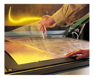
Fig. 1.2-27 Positioning of the film assembly in the copying frame for platemaking (Heidelberg)
