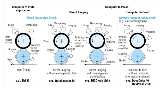
Fig. 4.4-2 Printing unit equipment in computer to press/direct imaging systems compared to off-line platemaking and computer to print
