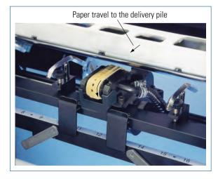
Abb. 2.1-53 Sheet slow-down device (Speedmaster SM 74, Heidelberg)
