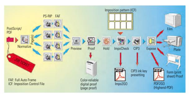
Fig. 3.2-90 Example of a dynamic workflow: Brisque, Scitex
