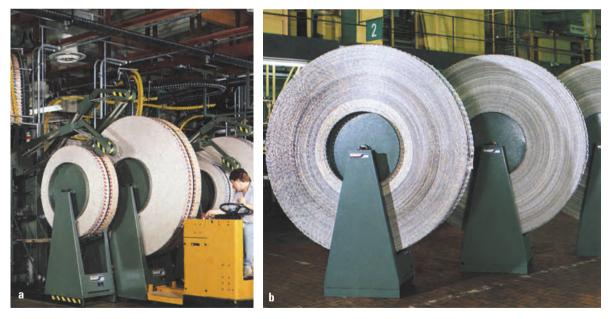
Fig. 7.3-7 Temporary storage for folded sheets on reel storage units (disk).
