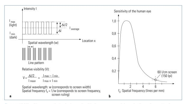
Fig 1.4-26 Visibility of line structures for the visual perception of the human eye at normal observation distance (approx. 30 cm). a Relative visibility of intensity variations (definition);
