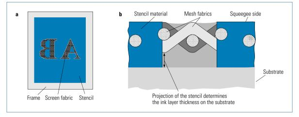
Fig. 2.4-3 Printing plate: screen with stencil.
