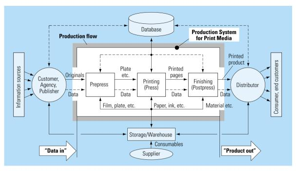
Fig. 9.2-12 Workflow for producing printed products as the basis of a digital, integrated production system for "data in", "product out"
