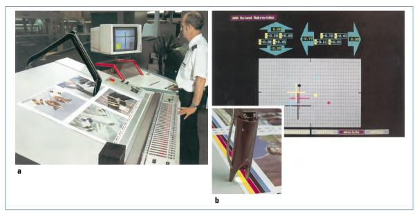
Fig. 2.1-139 "Video magnifying glass" for color register measurement and control.
