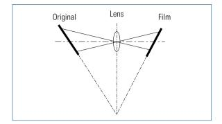
Fig. 3.1-20 Camera position to avoid plummeting lines
