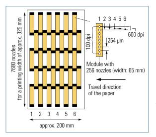
Modular structure (in principle) of a page-wide ink jet array by means of adjacent modules at right angles to direction of printing and increased resolution by means of successively positioned modules (Heidelberg/Spectra)
