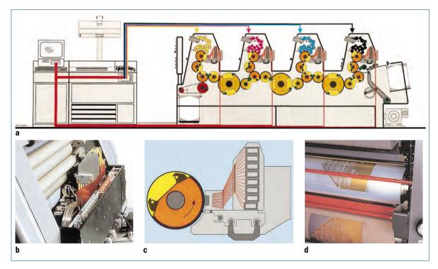
Fig. 4.4-4 Computer to press/direct imaging multicolor press.
