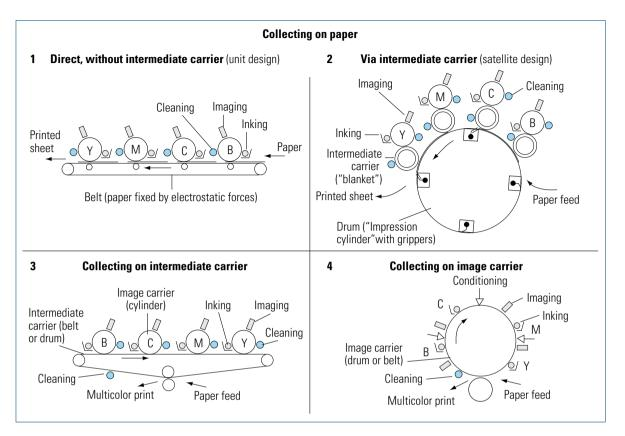
Fig. 4.5-16 Designs for collecting color separations in multicolor printing with computer to print systems (singlepass systems)
