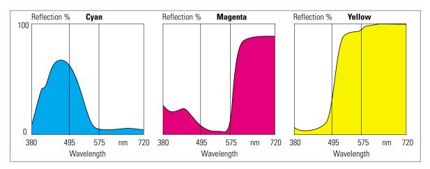
Fig. 1.4-22 Spectral distribution (degree of spectral reflection) of printing inks for multicolor printing [1.4-1]
