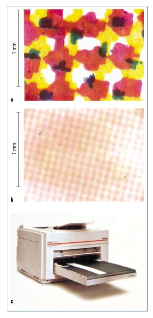
Fig 5.6-6 Printed dots produced by thermography.
