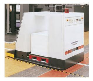
Fig. 8.1-12 Automated guided vehicle (AGV) for paper pile conveyance (Heidelberg/Eisenmann)
