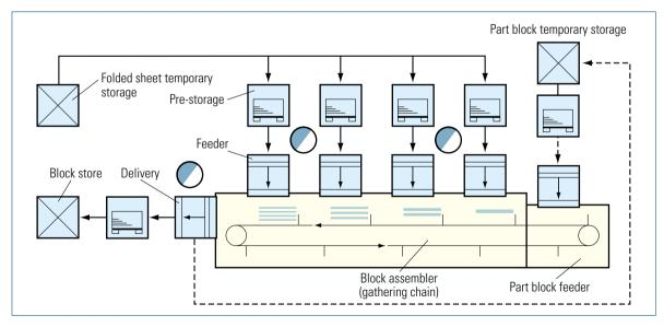
Fig. 7.2-49 Structure of a gathering machine (collating individual sheets or signatures)
