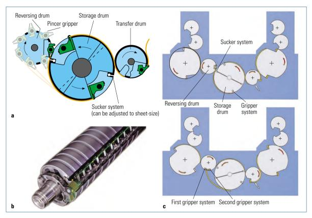
Fig. 2.1-49 Sheet reversing systems (three-drum system).
