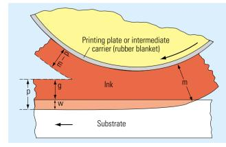
Approximation formula according to Walker-Fetzko for the transfer of ink from the printing plate (or intermediate carrier) onto the substrate
