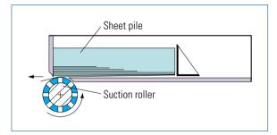
Fig. 7.2-33 Principle of the box/suction feeder
