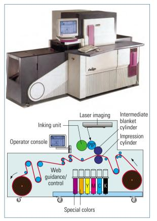
Computer to print system for multicolor printing on flexible web materials by collecting color separation images on intermediate cylinder and the subsequent transfer onto the web in one printing contact ("one shot" technology), (Omnius, Indigo)
