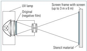
Fig. 2.4-7 Direct UV projection for screen printing stencil exposure
