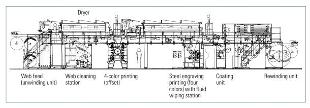
Fig. 2.5-12 Combined offset printing and steel engraving printing web-fed press for the reel-to-reel production of stamps (KBA)
