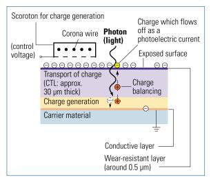
Structure of a coating of organic photoconducting material (OPC); a scorotron unit is shown for applying a homogeneous charge to the surface
