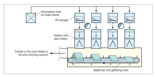
Fig. 7.2-55 Structure of a gatherer for single-layer blocks
