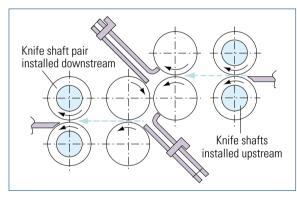
Fig. 7.2-27 Knife shafts in a buckle plate folding unit
