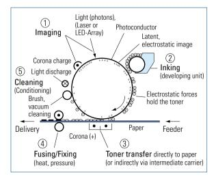
Fig. 5.2-1 Basic principle of electrophotography
