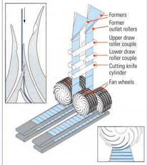
Fig. 2.1-101 Fan wheels dividing the product stream (Heidelberg)
