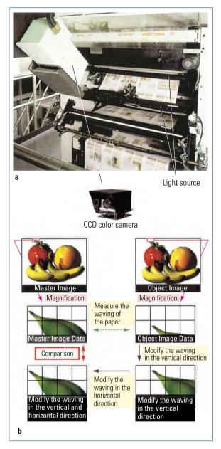
Fig. 2.1-140 Image inspection system on a web offset press.
