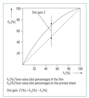
Fig. 3.1-31 Print characteristic curve and Dot gain
