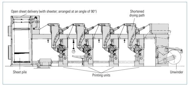
Fig. 2.2-9 Diagram of a gravure proof press with four printing units (fig. 2.2-8), unwinding unit and open sheet delivery (KBA)
