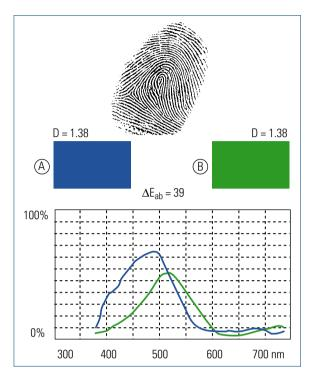
Spectral intensity distribution as a "fingerprint" on the example of two colors (A) and (B) (at the same optical density) [1.4-2] (Note: The colors in fig. 1.4-12 and fig. 1.4-13 may not be rendered accurately, they should only illustrate the problem in general)
