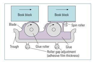
Fig. 7.2-67 Two-roller gluing unit [7.2-4]
