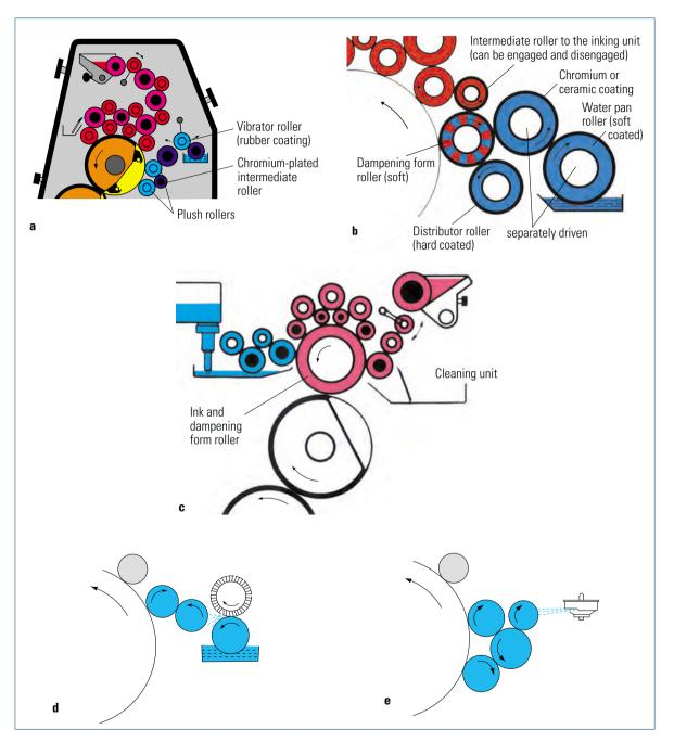
Fig. 2.1-15 Dampening system designs.
