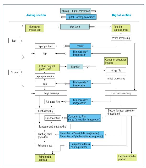
Fig. 3.1-10 Prepress workflow (analog and digital technologies)
