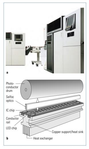
Printing system for double-sided printing on web material. **a** Twin installation of two systems for perfecting via turning bars; **b** Underlying principle of LED array for imaging (600 dpi), (DemandStream 8000 DI, Océ)
