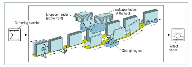
Fig. 7.2-46 Endpaper gluing machine in binding lines
