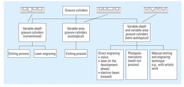
Fig. 1.3-11 Overview of the production of gravure cylinders
