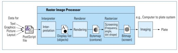
Fig. 3.2-44 PostScript-RIP in the prepress workflow
