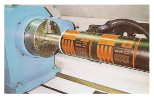
Fig. 2.3-10 Laser exposure of a sleeve printing master (digiflex, BASF)
