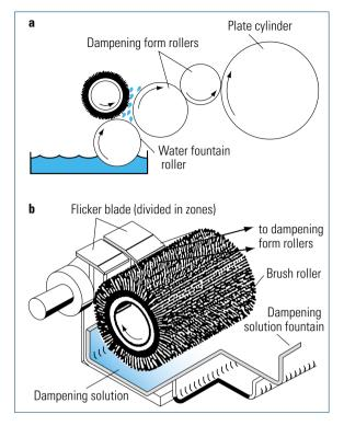
Fig. 2.1-107 Brush-type dampening system. a Brush for catapulting the solution from the fountain roller onto the form roller;
