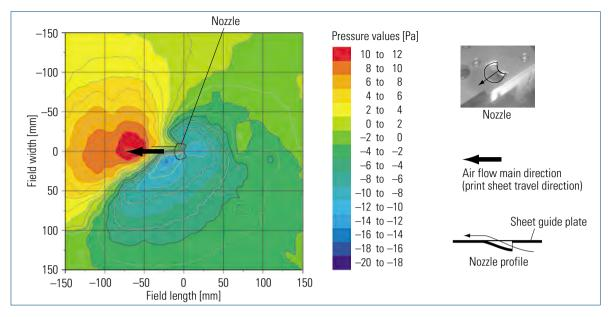
Fig. 13.1-54 Color chart of the measured pressure field on the nozzle and its surrounding on a sheet guide plate (Heidelberg)
