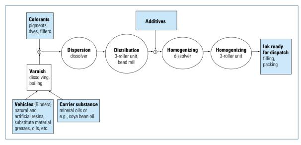
Fig. 1.5-10 Producing ink for sheet-fed offset printing
