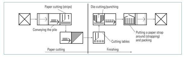
Fig. 7.3-11 Diagram of a module configuration for die-cut labels
