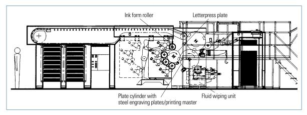
Fig. 2.5-6 Orlof steel engraving unit for one-sided printing, including a fluid wiping unit (Super-Intagliocolor 212, KBA)
