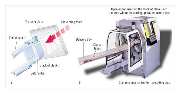
Fig. 7.2-14 Column die-cutter in horizontal construction. a Schematic structure of the die-cutting tool;
