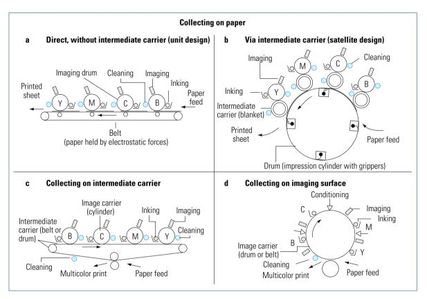
Fig. 5.1-13 System concepts with several printing units for collecting color separations for multicolor printing (singlepass system)
