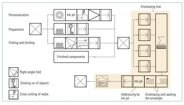
Fig. 7.3-15 Mailing production line for product sections with a high presentation requirement
