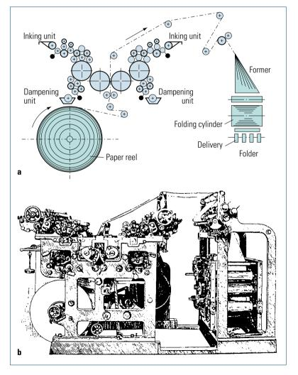
Fig. 13.1-8 Web offset press based on Caspar Hermann's patent made by VOMAC, around 1916
