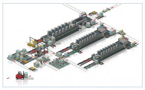
Fig. 8.1-14 Overview of a paper pile logistics system for feeding and removing paper piles for several sheet-fed presses (MAN Roland)
