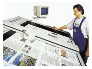
Fig. 2.1-133 Scanning densitometer for two-dimensional measurement positions on the printed sheet (Densitronic, KBA)
