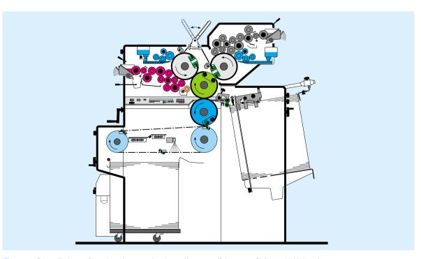
Fig. 1.6-7 Four-cylinder configuration of a two-color sheet offset press (Printmaster QM 46-2, Heidelberg)
