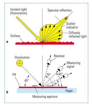
**Fig. 1.4-57** Basic principle of gloss measurement. **a** Reflection behavior of a rough surface;
