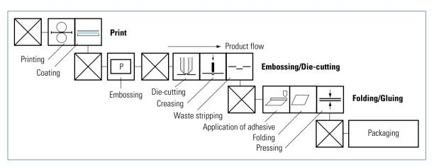
Fig. 7.3-39 Technology for the production of folding boxes
