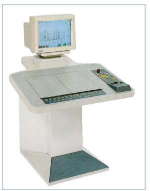
Fig. 2.1-94 Control console with monitor (touch screen), ink zone and color register control functions (Ewert Ahrensburg Electronic)
