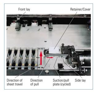
Fig. 2.1-31 Pneumatic pull lay (KBA)
