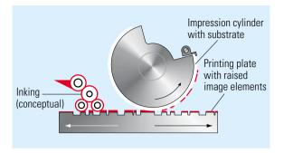
Fig. 1.3-7 Letterpress (schematic diagram)
