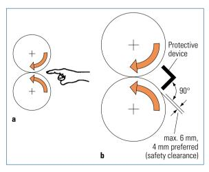
Fig. 13.2-3 Danger zone of moving rollers and safety measure. a Danger zone at the roller infeed (infeed gap);
