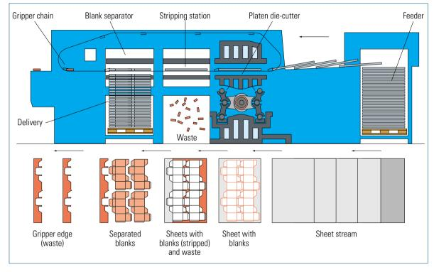
Fig. 7.2-17 High-speed die-cutter (Bobst)
