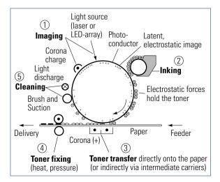
Fig. 1.3-27 The basic structure of electrophotography
