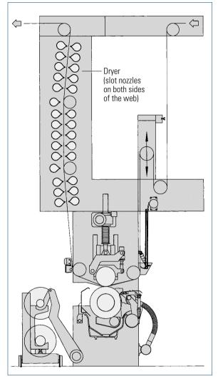
Dryer with slot nozzles. The paper web is blasted with air on the front and reverse side from the slot nozzles because some of the solvent penetrates through the paper to the reverse side. The arrangement of the dryer is single-sided with regard to the printing unit (KBA)
