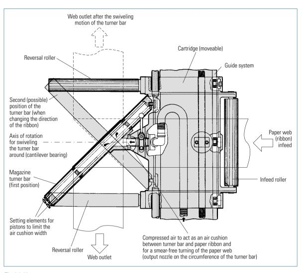
Magazine turner bar in the superstructure with cantilever bearing arrangement; the turner bar can be used in two positions (KBA)
