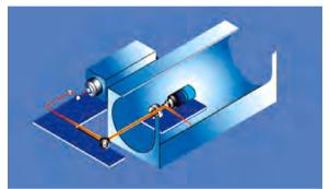
Fig. 4.3-6 Internal drum and beam path in a plate imagesetter (PlateRite Pl-R2080, Dainippon Screen)
