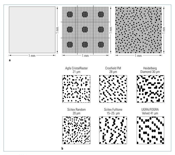
Fig. 1.4-37 Digital screen structure.
