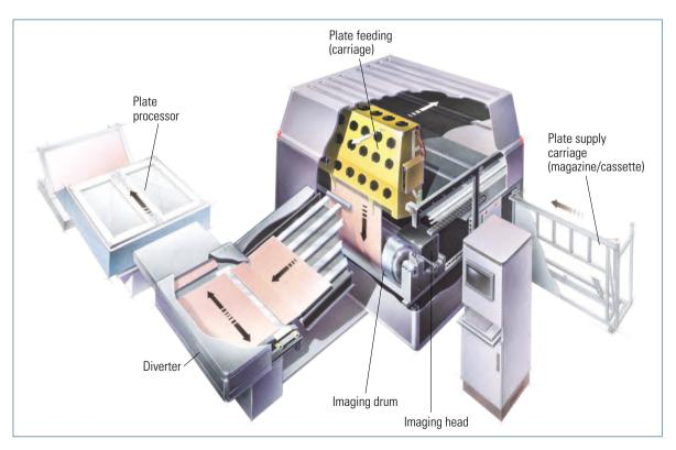
Fig. 4.3-18 Diagram of a fully automated computer to plate system (Platesetter 3244, Heidelberg/Creo)
