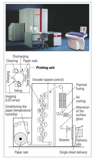
Computer to print multicolor printing systems for double-sided printing on web material (electrophotography, LED imaging, powder toner) (DCP/32D, Xeikon; diagram drawn up using company literature)
