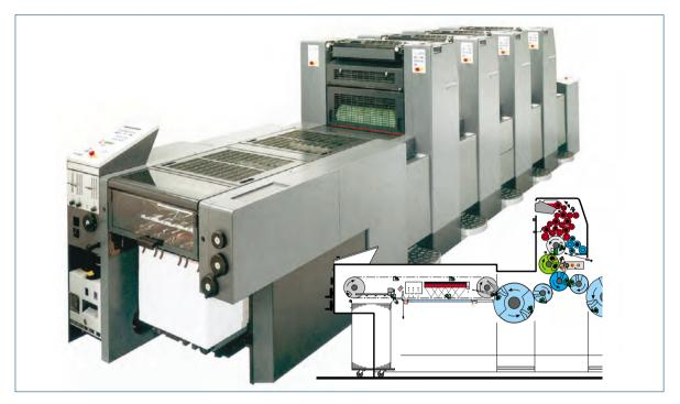
Speedmaster SM 52, 4-color press, 2/2 sheet reversal, high-pile delivery; sheet size 370 mm × 520 mm, printing speed 15000 impressions/ hour (Heidelberg)
