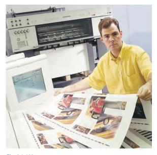
Printed sheet taken from the delivery of a sheet-fed offset press for quality control purposes (Heidelberg)
