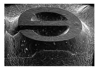
Fig. 3.1-52 Microphoto of a letterpress plate
