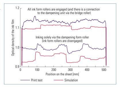
the ink layer thicknesses running out at the nip; see also sec. 2.1.1.3, fig. 2.1-8) for the simulation program developed by Patzelt and Ruder [13.1-13].
