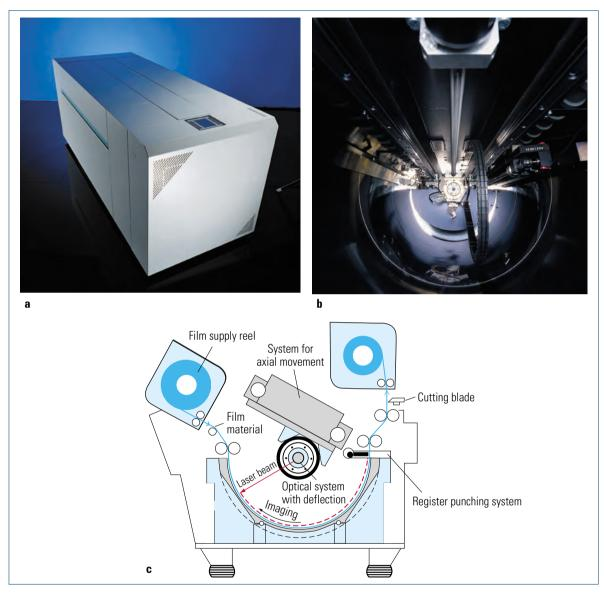
Fig. 4.2-2 Computer to film equipment for full-sheet film output.
