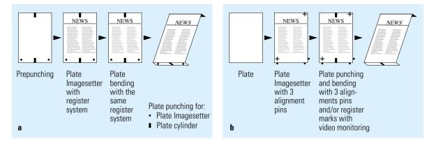
Fig. 8.1-3 Exposure with computer to plate technology and plate bending. a Pre-punched plate:
