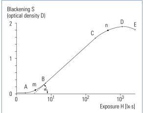
Fig. 3.1-15 Blackening curve (gradation curve)
