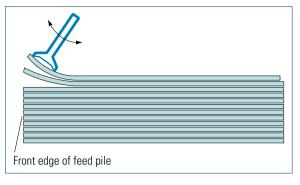
Fig. 2.1-26 Sheet separation by sucker tilting
