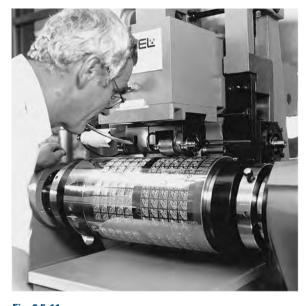
Fig. 2.5-11 Die-transferring machine for producing steel engraving cylinders for postage stamp printing (Goebel)
