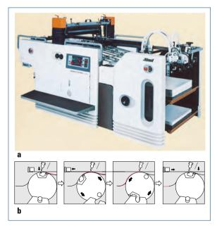
Fig. 2.4-17 Cylinder screen printing press (flat-round). a Printing system (model: Maestro, Sakurai); b The printing sequence
