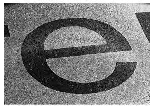
Fig. 3.1-47 Microphoto of an offset plate surface
