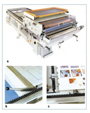
**Fig. 3.1-45** Flat-bed offset proofing press (Korrex 2000, FAG). **a** Proofing press;
