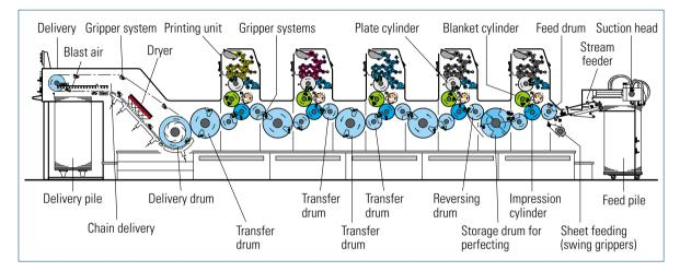
Fig. 2.1-18 Sheet conveyance in a sheet-fed offset press in unit design (Speedmaster SM 74-5-P-H, Heidelberg)
