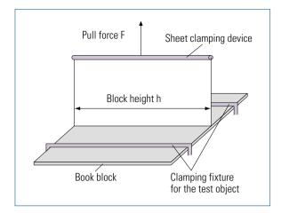
Fig. 7.2-70 Pull test
