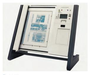
**Fig. 2.1-162** Plate image reader for determining the zonal ink requirement of an offset printing plate for ink feed presetting (CPC 31, Heidelberg)
