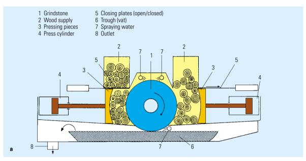
Fig. 1.5-1 Production of groundwood pulp. a Principal structure of a magazine grinding unit;
