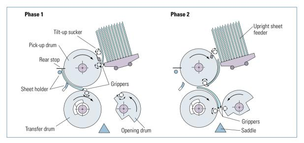
Fig. 7.2-56 Feeder for gatherers based on the transfer technique (Heidelberg)
