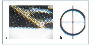
Fig. 1.4-54 Color register deviations. a Halftone multicolor image; b Register measuring mark
