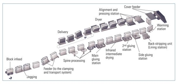
Fig. 7.2-65 Diagram of a perfect binding machine (Ratiobinder, Kolbus)
