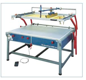
Fig. 2.4-12 Flat-bed screen printing equipment (Siri/Steinmann)
