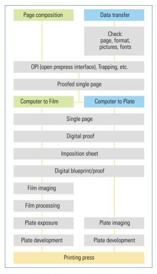
Fig. 3.2-88 Workflow in computer to film and computer to plate
