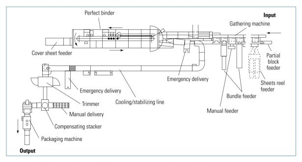
Fig. 7.3-24 Outline plan of equipment for finishing magazines (e.g., trade/hobby magazines)
