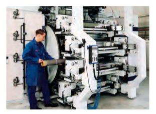
Fig. 2.3-17 Change of a flexographic plate cylinder sleeve (Fischer & Krecke)
