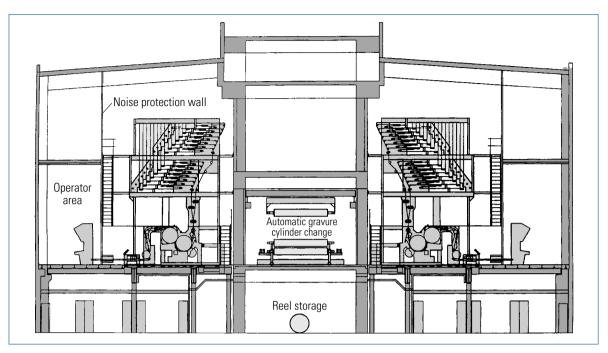
Fig. 2.2-27 Parallel arrangement of two gravure printing presses with a central device for automatic gravure cylinder change (KBA)
