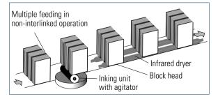
Fig. 7.2-78 Edge coloring machine, head trim (Kolbus)
