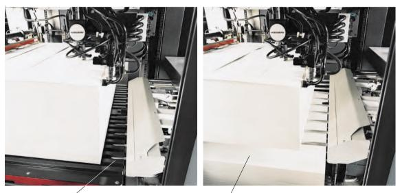
**a** Rake moves beneath the pile (residual pile)
