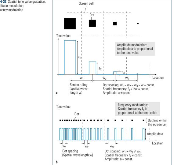
Fig. 1.4-32 Spatial tone value gradation. a Amplitude modulation: **b** Frequency modulation
