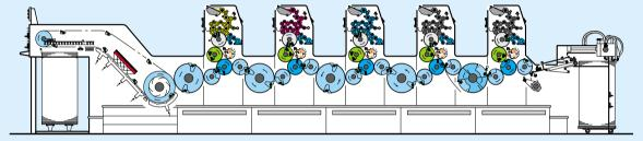
Fig. 1.3-21 Typical example of a sheet-fed offset press (Speedmaster SM 74-5-P-H, Heidelberg)
