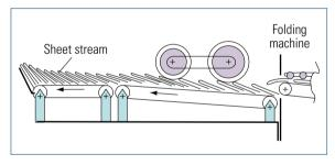
Fig. 7.2-34 Stream delivery on a folding machine
