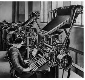
Fig. 13.1-30 Blower lead typesetting machines.
