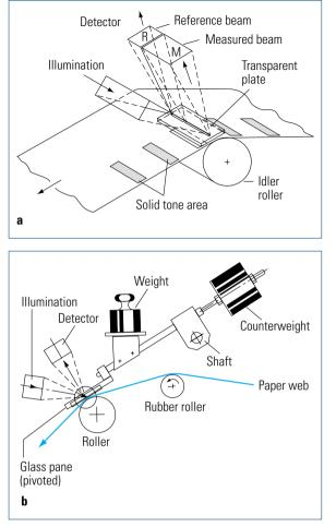
Fig. 1.7.17 Dynamic drying test device.
