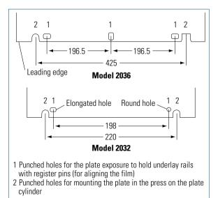
Fig. 3.1-41 Plate punch (CONTROL 2000 register system, Bacher)
