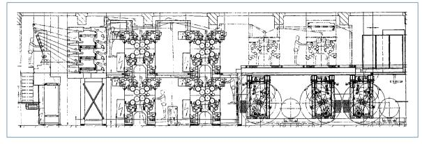
Fig. 2.1-196 Four-high units (compact design) and arch-type printing units in newspaper printing (IFRA/KBA)
