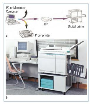
Fig. 4.4-20 Computer to press/direct imaging in screen printing. a Workflow;
