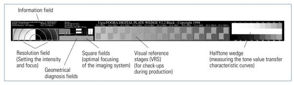
Fig. 4.3-19 Digital plate control wedge (Ugra/FOGRA)
