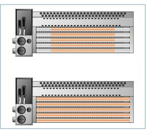
Fig. 2.1-60 Adapting the radiation width to the print format (Drystar, Heidelberg)
