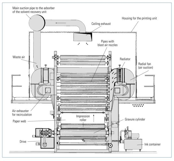
Cross-section of a gravure printing unit with the significant elements for drying (high velocity nozzle dryers). The stream of air through the nozzle pipes in the center is fed by two radial fans, located at the side (KBA)
