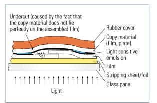
Fig. 3.1-38 Undercutting caused by overlapping films
