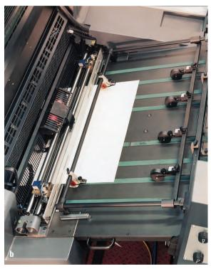
**Fig. 2.1-24** Stream feeder. **a** Diagram of the sheet transportation; **b** Evample of a sheet stream feeder (Hei
