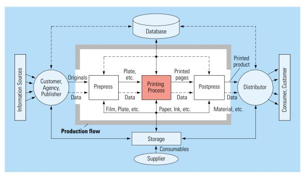
Fig. 1.2-31 The printing process in the production flow for printed products
