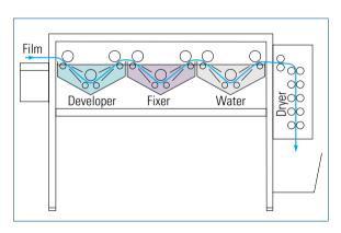
Fig. 3.1-25 Film developer in tray design [3.1-9]
