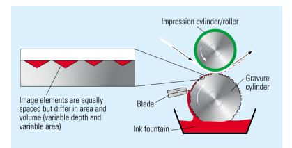
Fig. 1.3-10 Gravure printing (schematic diagram)
