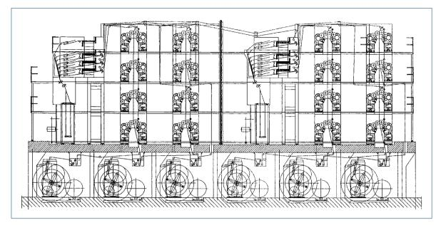
Fig. 2.1-199 Web-fed printing system with four-high units in the form of stacked arch-type printing units (IFRA/KBA)
