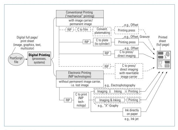
Fig. 8.2-11 Digital printing: processes, components, and systems
