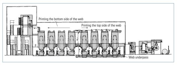
Fig. 2.2-29 Gravure printing press with reel stand and folder on the same floor (KBA)
