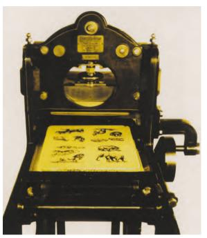
Fig. 1.3-17 Stone lithographic press (manually operated)
