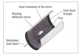
Fig. 3.1-7 Internal drum film imagesetter (AGFA)
