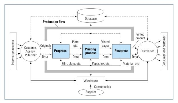
Fig. 8.2-1 Production flow (prepress, press, postpress) with material and data flow for the production of printed products
