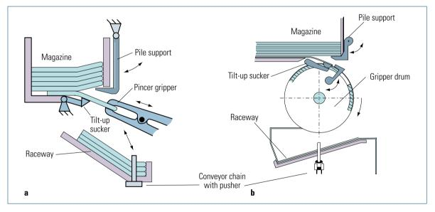
Fig. 7.2-51 Feeder variants in gathering machines. a Feeder with pincer grippers; b Feeder with gripper drum
