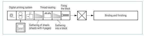
Fig. 7.3-32 Finishing operations for thread-sealed blocks
