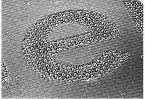
Fig. 3.1-54 Microphoto of a screen printing master/plate (stencil shown at the top/squeegee side, printing substrate underneath)
