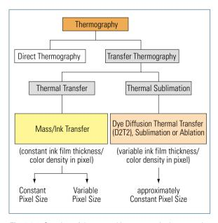
Fig. 5.6-1 Overview of thermographic processes in thermography
