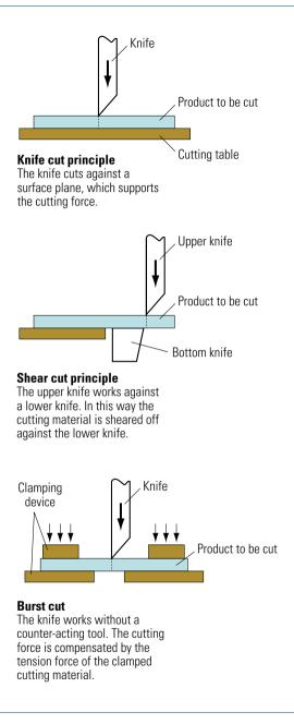
Fig. 7.2-2 Cutting principles
