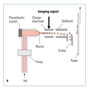
Fig. 5.5-2 Functioning principles for ink jet technologies.
