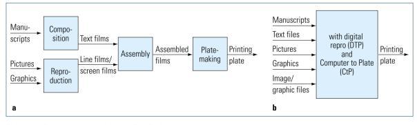
Fig. 1.2-30 Evolution in prepress through digitalization of the processing sections.
