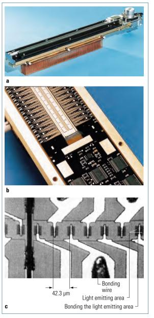
Design of an LED array for imaging in an electrophotographic printing system.
