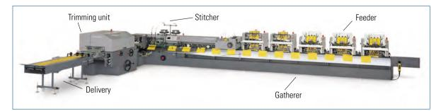
Fig. 7.2-58 Wire-stitching production line/gatherer-stitcher (Stitchmaster ST 250, Heidelberg)
