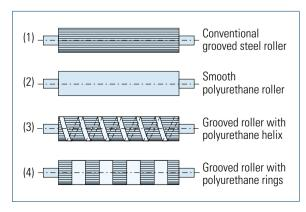
Fig. 7.2-24 Types of folding rollers with homogeneous and composite surfaces
