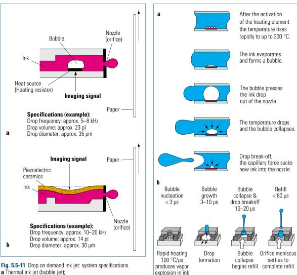
a Thermal ink jet (bubble jet); **b** Piezo ink jet
