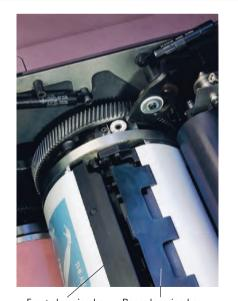
Front clamping bar Rear clamping bar
