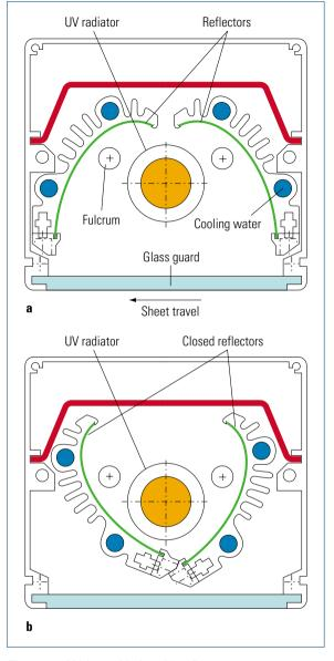
Fig. 2.1-61 UV dryer with shuttable reflectors. a Open reflector; b Closed reflector (Dr. Hönle)
