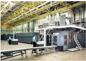
Fig. 1.2-36 Web-fed offset printing system (M-600, Heidelberg)
