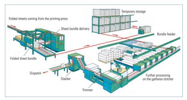
Fig. 7.3-6 Logistics system for folded sheet bundles for producing magazines (Müller Martini)
