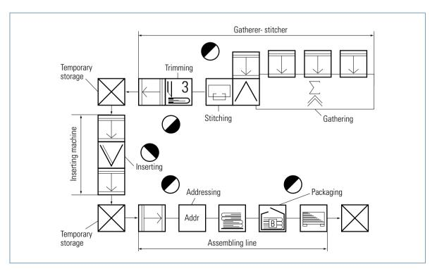
Fig. 7.3-25 Magazine production with technically separate (unlinked) modules
