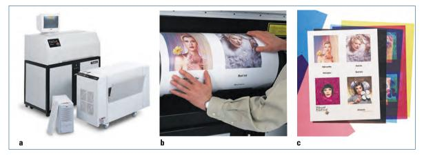
Fig. 3.2-77 Screen proof ("True proof") with thermal transfer on production paper (job paper).
