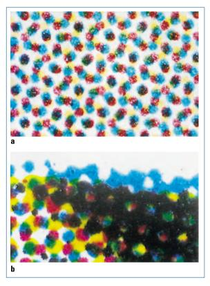
Autotypical multicolor printing (microscopic photo of a print image section); scale: cell spacing about 167 µm.
