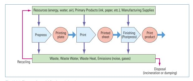
Fig. 13.2-1 Diagram of material flow in a printing plant
