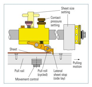
Fig. 2.1-30 Pull lay for lateral sheet alignment
