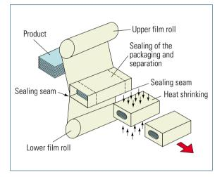
Fig. 7.2-99 Tubular sleeve wrapping with two seams
