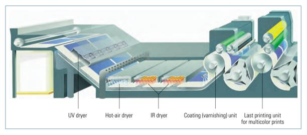
Fig. 1.7-2 Installation of different types of drying systems in a sheet offset press (Speedmaster CD, Heidelberg)
