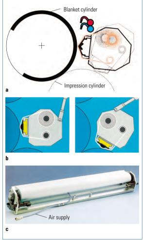
Fig. 2.1-153 Convertible cleaning system with washing cloth.
