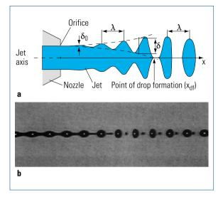
Fig. 5.5-6 Drop formation with continuous ink jet.
