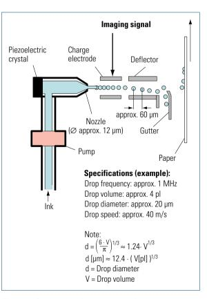
Fig. 5.5-5 Continuous ink jet: process specifications
