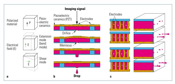
Fig. 5.5-13 Structure of drop on demand ink jet systems using piezoelectric ceramics.
