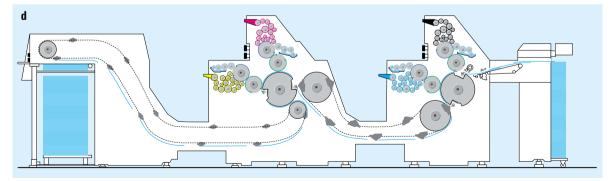
Fig. 1.6-5 Design concepts and cylinder configurations for multicolor sheet-fed offset printing presses.
