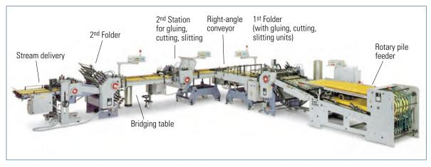
Fig. 7.3-16 Finishing line (Flexomailer; Heidelberg)
