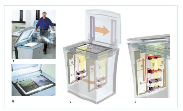
Fig. 3.2-30 Flat-bed scanner.
