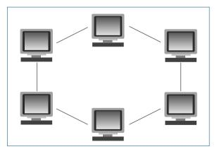
Fig. 3.2-56 Ring structure of a network
