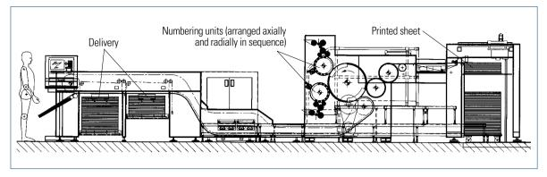
Fig. 2.5-8 Numbering machine for security printing (Super-Numerota, KBA)
