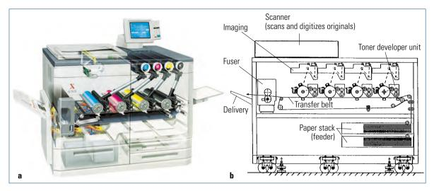
Fig. 1.3-28 NIP printing system (electrophotography) for multicolor printing.
