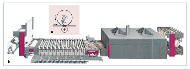
Fig. 2.4-19 Screen printing system for multicolor textile printing.
