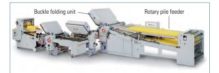
Fig. 7.2-30 Combined folding machine with buckle folding and knife folding systems and vertical pile feeder (Proline KI 55, Heidelberg)
