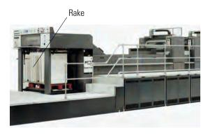
Fig. 8.1-10 Delivery with equipment (rake, etc.) for semi-automatic pile change in non-stop operation (Heidelberg)
