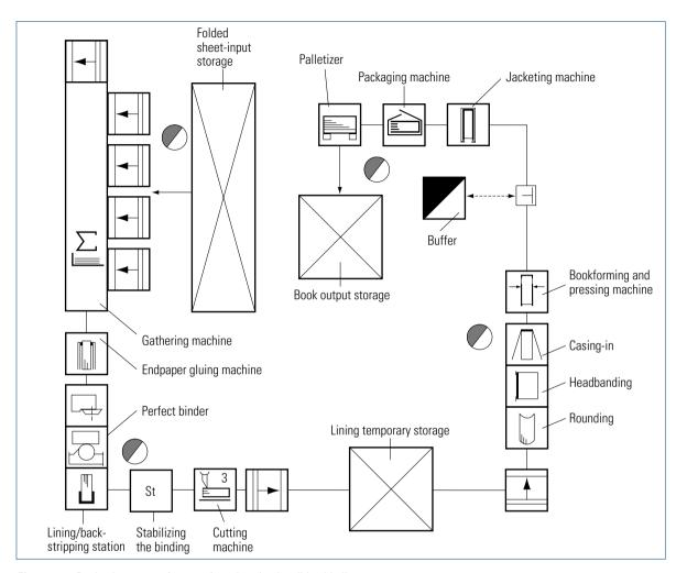
Fig. 7.3-28 Production system for manufacturing simple edition bindings
