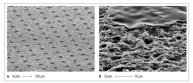
**Fig. 2.1-3** Aluminum printing plate with halftone dots. **a** Magnified a hundred times;
