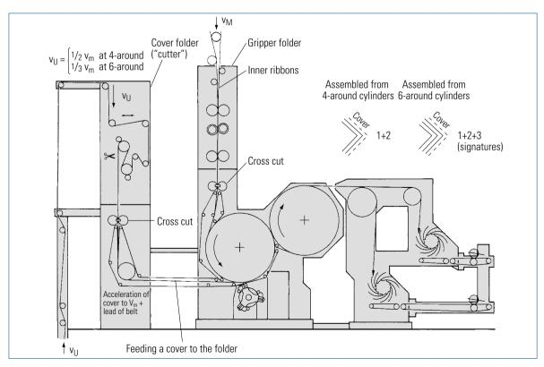
Fig. 2.2-22 Devices for feeding covers to a gripper folder (KBA)
