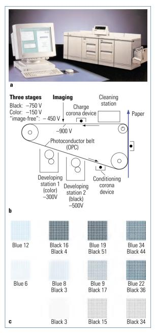
Electrophotography with tri-level system for printing special colors and highlight color.
