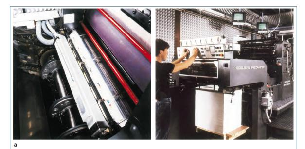
In-line color density measuring systems. **a** In-line color densitometer for use with print control strips on the impression cylinder of the last printing unit in a sheet-fed offset press (Reprotest);
