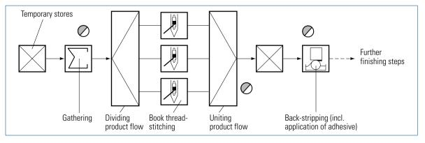
Fig. 7.2-63 Basic principle of thread-stitching lines
