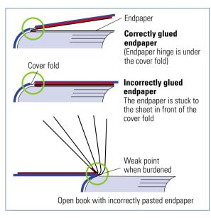
Fig. 7.2-48 Tension due to incorrect endpaper gluing
