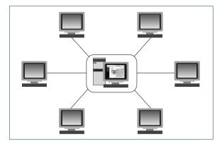
Fig. 3.2-54 Star structure of a network
