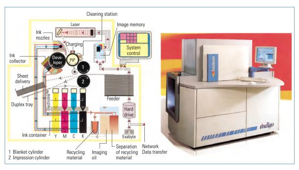
Computer to print system for multicolor printing (electrophotography, ROS laser imaging, liquid toner, intermediate cylinder) with the option of sheet turning for double-sided (duplex) printing (E-Print 1000/TurboStream, Indigo; see also fig. 4.1-7)
