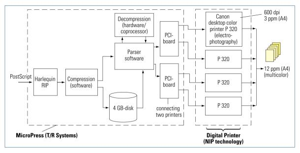
Fig. 9.2-4 Clustered printing system (MicroPress/P320, T/R Systems/Canon)
