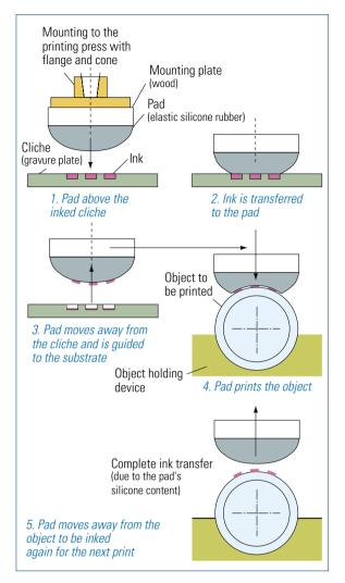
Fig. 2.5-31 Schematic diagram of pad transfer printing
