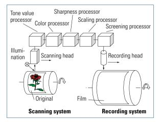
Fig. 3.1-35 Schematic diagram of a color separation scanner
