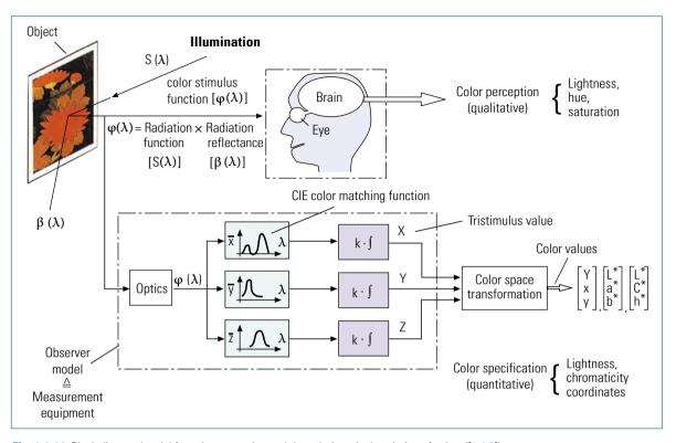
Fig. 1.4-14 Block diagram/model for color perception and the colorimetric description of colors ([1.4.2])
