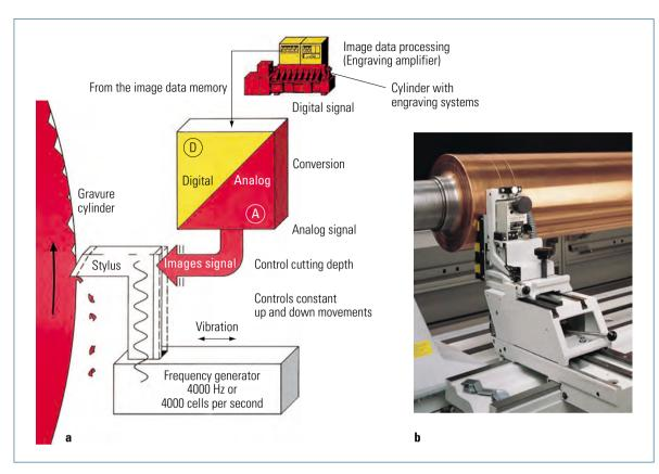
Fig. 1.3-15 Cylinder engraving with stylus.
