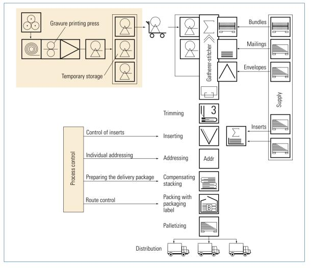
Fig. 7.3-22 System for processing mass-circulation magazines
