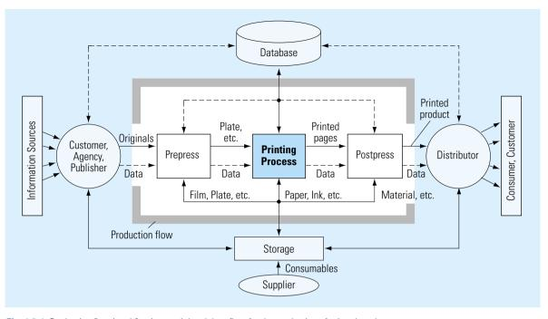
Fig. 1.3-1 Production flow (workflow), material and data flow for the production of printed products
