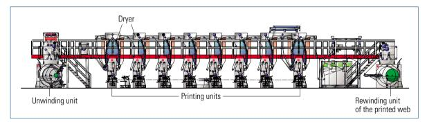
Fig. 1.6-18 Gravure printing press, eight printing units, unit design (W&H)
