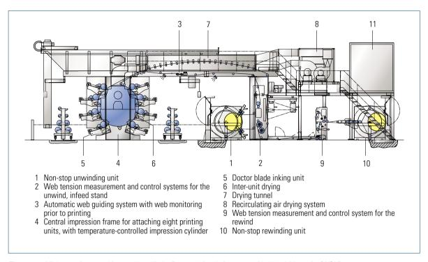
Fig. 1.6-23 High-capacity central impression cylinder flexographic printing press with eight inking units (W&H)
