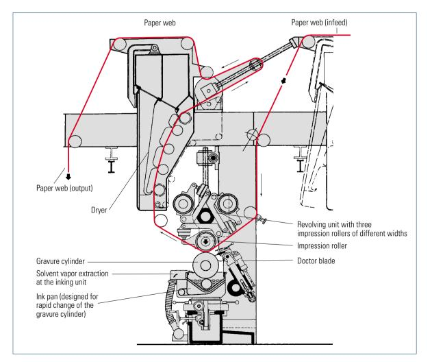
Fig. 2.2-8 Structure of a gravure proof press unit (KBA)
