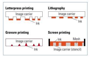
The four main conventional printing technologies (in principle)
