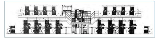
Fig. 2.1-195 Vertical configuration of printing systems above one another for multi-web newspaper printing (IFRA/Solna)
