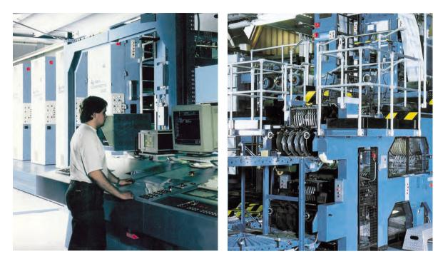
Web offset printing press (16 pages, max. 80000 copies/hour) with central control console and modular folder with two deliveries (Compacta 218/folder P3, KBA)
