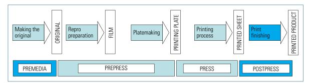
Fig. 3.1-1 The production of film and printing plate within the process chain for producing print media
