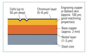
Fig. 1.3-12 Structure of a gravure cylinder
