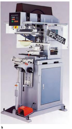
Fig. 2.5-34 Single-color pad transfer printers.
