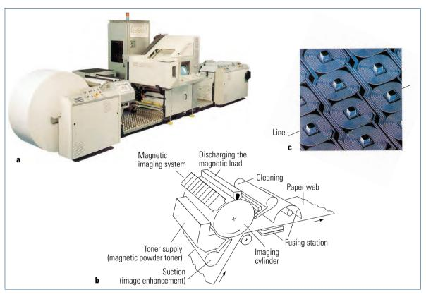
Fig. 4.5-13 Digital printing system (magnetography) for printing on web material.
