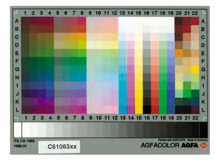
Fig. 3.2-64 Test image according to ISO 12641 (input test image)
