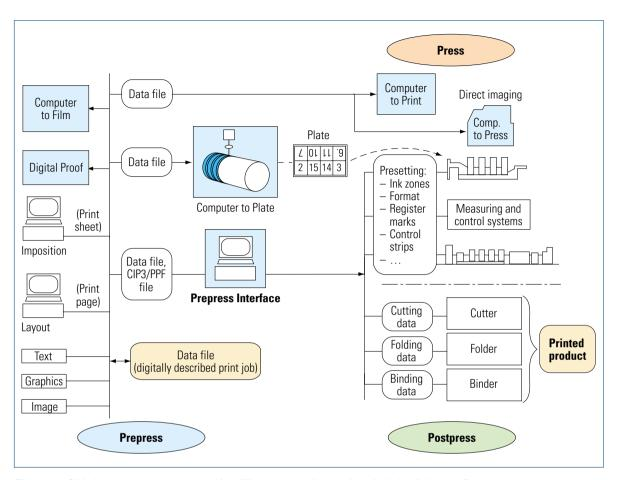
Fig. 10.3-2 Digital process control and networking different means of production within the digital workflow
