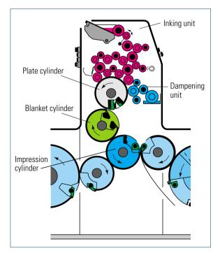
Fig. 1.3-19 Typical sheet-fed offset printing unit
