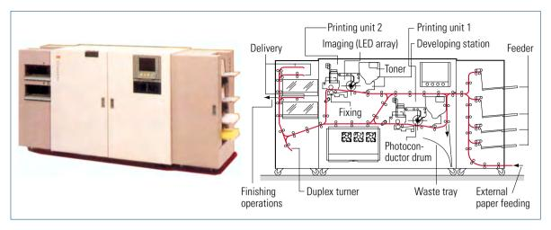
Printing system for double-sided single-color printing on sheet material (electrophotography with LED imaging, powder toner) with two printing units (DemandStream 4000 DI, Océ)
