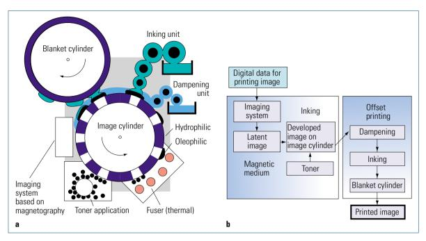
Fig. 4.4-29 Magnetolithography: concept for imaging an offset plate through magnetic fields, powder toner, and heat fusing. a Principle for platemaking (erasing system is not shown);
