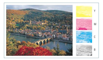
serves as the image carrier for the offset press. In every printing technology a plate must be produced for each color to be printed.
