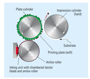
Fig. 2.3-2 Flexography (the principle of the process)
