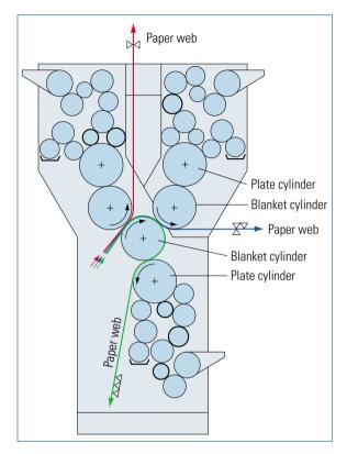
Fig. 2.1-118 Y-type printing unit (KBA)
