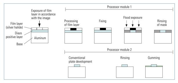
Fig. 4.3-23 The imaging and developing of multi-layer printing plates (sandwich plates), for example, Polychrome CTX plates
