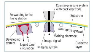
Fig. 5.7-2 Imaging and inking process in electrography
