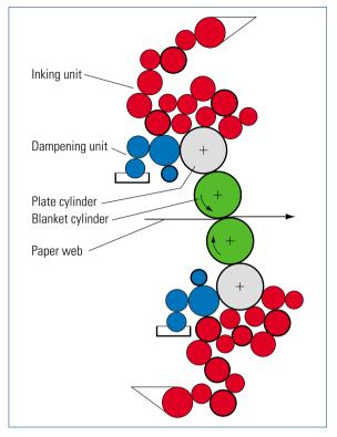
Fig. 2.1-103 Blanket-to-blanket printing unit of a web offset press (M-600, Heidelberg)
