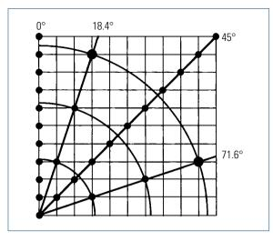
The screen angle and screen frequency of rational screens deviate from the ideal screen ( $18.4^{\circ}$  instead of the ideal  $15^{\circ}$  and  $71.6^{\circ}$  instead of the ideal  $75^{\circ}$ ; screen frequency see table 3.2-1)
