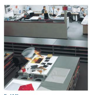
**Fig. 1.2-24** Prepress with conventional film stripping and digital master preparation (text, images, graphics) with EDP systems
