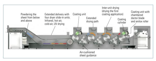
Fig. 2.1-65 Off-line surface finishing system (Speedmaster CD 102 LYYL, Heidelberg)
