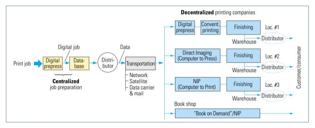
Fig. 4.1-14 Decentralized production of print media by applying Computer to ... technologies
