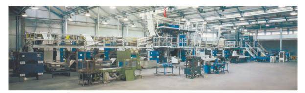
Examples of installations of a web offset newspaper printing system (Model line for max. web width of 1020 mm, cut-off max. 630 mm; for coldset max. 45000 copies/hour, for heatset max. 35000 copies/hour) (Mercury, Heidelberg)
