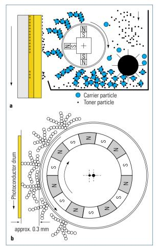
Magnetic brush for toner transfer to the photoconductor drum. a Carrier and toner particles in the developer station with transfer by magnetic roller; stationary magnets, roller shell rotates; **b** Magnetic brush design for smooth transfer of the toner to the photoconductor surface; magnetic roller and application roller turn in opposite directions (Kodak)
