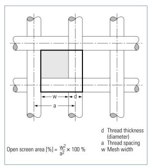
Fig. 2.4-4 The screen geometry
