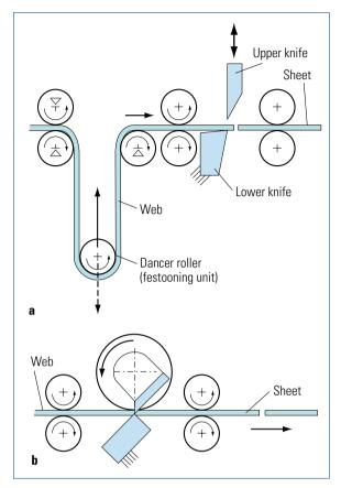
Fig. 7.2-10 Structure of cutters. a Cross cutter; b Rotary cross cutter
