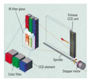
Color image scanning using three sensor lines with RGB color filters; scan motion for image recording via stepper motor and spindle (AGFA)
