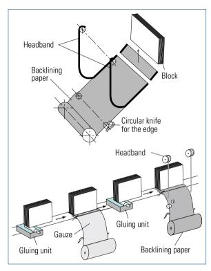
Fig. 7.2-84 Principle of headbanding by machine (Kolbus)
