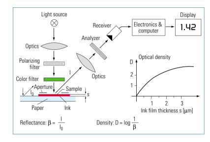
Fig. 1.4-43 The basic principle of a densitometer for optical density measurement
