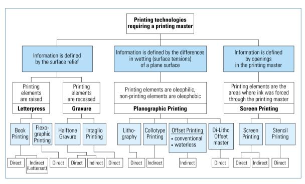
Fig. 1.3-3 Overview of printing technologies requiring a printing plate (master)
