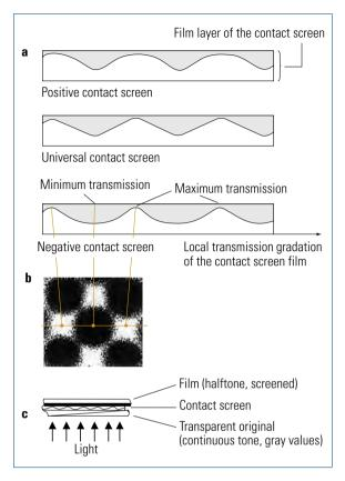
Fig. 3.1-30 Contact screen (schematic representation). a Density profile of various contact screen films; b Places of minimum and maximum transmission; c Layer arrangement in the vacuum frame
