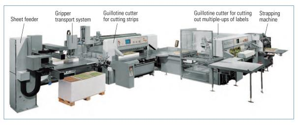
Fig. 7.3-10 Label cutting line (Polar Mohr)
