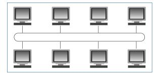
Fig. 3.2-55 Bus structure of a network
