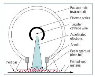
Fig. 1.7-13 Principle of electron-beam tube (MEC)
