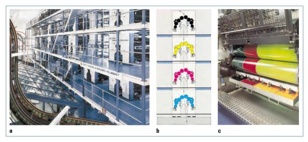
Web offset newspaper printing system with Anilox short inking units (web width max. 1680 mm, cut-off max. 578 mm, double-sized cylinder, max. 70000 copies/hour in double production).
