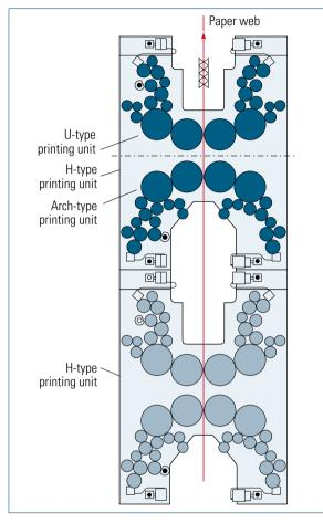
Fig. 2.1-120 Four-high unit composed of two stacked H-type printing units (GOSS)
