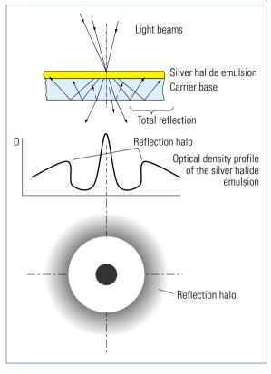
Fig. 3.1-17 Formation of the reflection halo by total reflection
