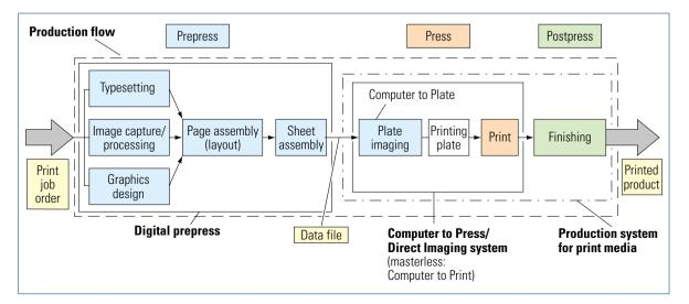
Fig. 10.3-1 Workflow (production flow) for the production of print media
