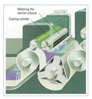
Fig. 2.1-62 Coating unit (Speedmaster 102, Heidelberg)
