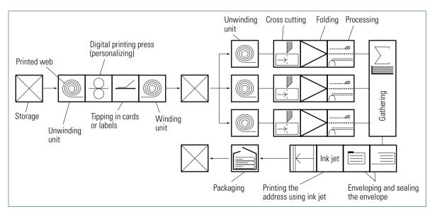
Fig. 7.3-14 Production line for mailings consisting of simple folded signatures
