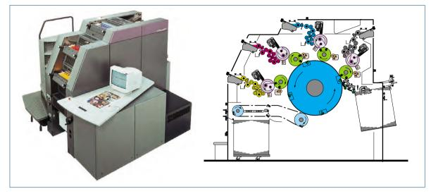
Fig. 4.4-8 Quickmaster DI computer to press/direct imaging system for multicolor printing in waterless offset (QM DI 46-4, Heidelberg)
