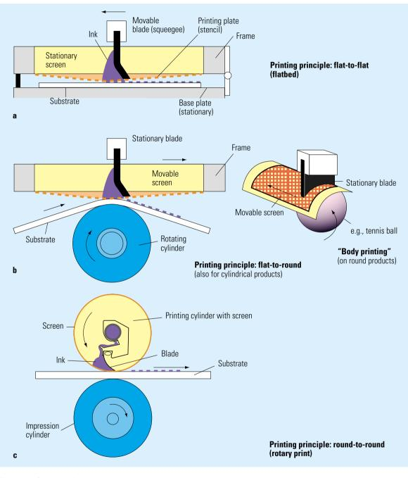
Fig. 1.3-24 Screen printing technologies.
