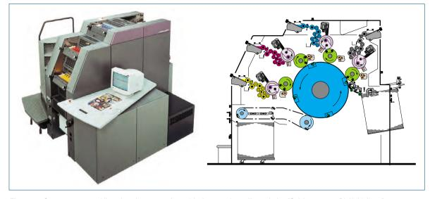
Fig. 4.1-5 Computer to press/direct imaging system for multicolor waterless offset printing (Quickmaster 46-DI, Heidelberg)
