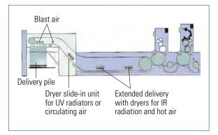
Fig. 2.1-57 Extended chain delivery with dryers (KBA)
