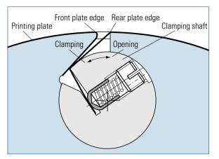
Fig. 2.1-105 Plate clamping mechanism (M-600, Heidelberg)
