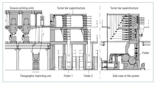
Fig. 2.2-31 Press installation with two folders alongside one another and an additional flexographic imprinting unit (KBA)
