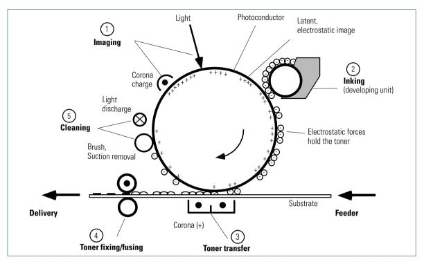
Fig. 1.5-12 Electrophotography (basic principle of the process)
