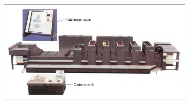
Multicolor sheet-fed offset press (with coating unit and extended delivery) and control console for remote press settings and production monitoring, and plate image reader for ink zone presetting (SM 102/CPC 31/DataControl, Heidelberg)
