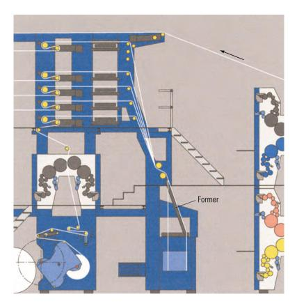
Fig. 2.1-88 Former. a Former on a web offset press (M-600, Heidelberg); b Former with 3 webs running in (IFRA)
