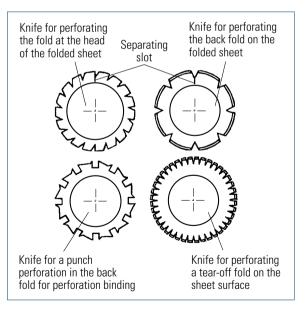
Fig. 7.2-28 Example of perforating tools for knife shafts
