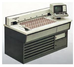
Scanning densitometer for color measurement and data transfer to the press control console for ink control in multi-machine operating mode (CPC 2, Heidelberg)
