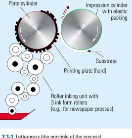
Fig. 2.3-1 Letterpress (the principle of the process)
