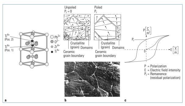
Fig. 4.4-32 Ferroelectric material for use as re-imageable surfaces with storage capability for direct imaging printing systems. a PZT (lead-zirconate-titanate) mixed crystal for building up ferroelectric coatings;
