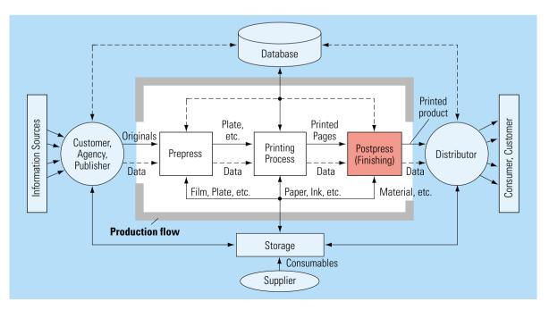
Fig. 1.2-37 Finishing processes in the production flow for printed products
