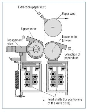
Slitting unit integrated in the superstructure of the gravure printing press (KBA)
