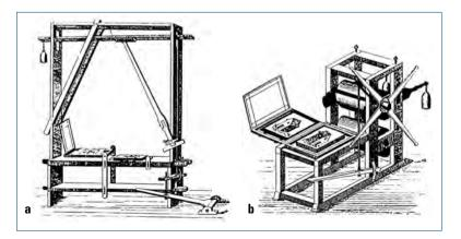
A lithographic automatic cylinder press with thrust crank drive from around 1815, such as continued to be used for a long time for art prints (posters). Operation involved 3 persons: one for driving the wheel (on the right), one for feeding the sheet, and one for catching the sheet (on the left, rear); the supervisor is standing in front
