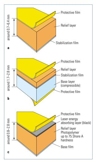
Fig. 2.3-7 Structure of the various flexographic plates.
