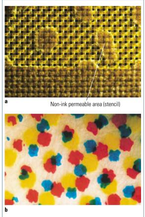
Fig. 1.3-23 Microphoto of screen printing. a Screen fabric with stencil; b Halftone dots of a three-color screen print
