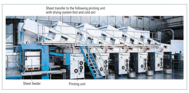
Fig. 2.2-34 Multicolor sheet-fed gravure printing press for printing of packaging material; diagram in figure 1.6-8 (Rembrandt 142, KBA)
