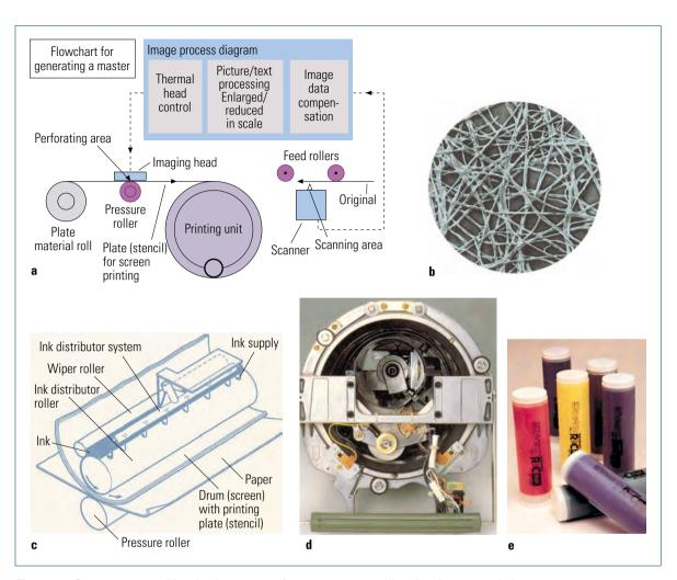
Fig. 4.4-19 System concept and functional components for computer to press/direct imaging screen printing systems.
