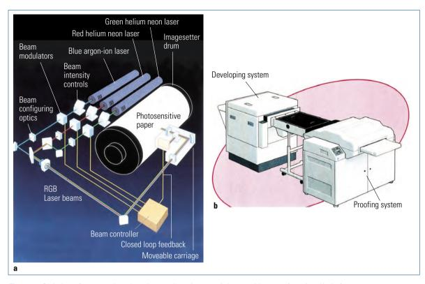
Fig. 5.8-1 Digital proofing system based on photography, using coated photographic papers (e.g., from Konica). a Imaging via laser systems making use of the external drum principle; resolution 2000 or 4000 dpi (adjustable), A2+ format; b Proofing system with developer (IntelliProof/Colorsetter 4400, Optronics/Intergraph; status: 1995)
