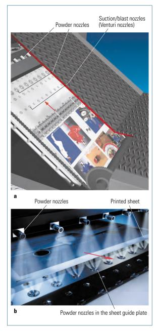
Fig. 2.1-56 Powder application in the delivery area.
