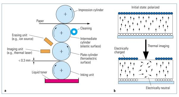
Fig. 4.4-34 Direct imaging with re-imageable plate cylinder.
