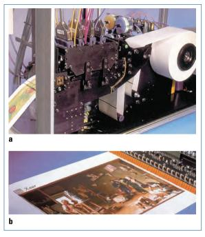
Fig. 5.5-28 Ink jet printing system for multicolor printing. a Laboratory system with piezo drop on demand ink jet print heads; b Project study on multicolor printing with modular structure, pagewide printing system (XAAR Digital)
