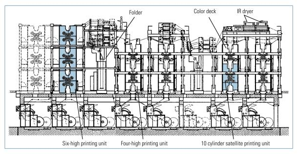
Web printing system combining 10-cylinder satellites, color decks and four-high units, extended to form six-high units (IFRA/WIFAG)
