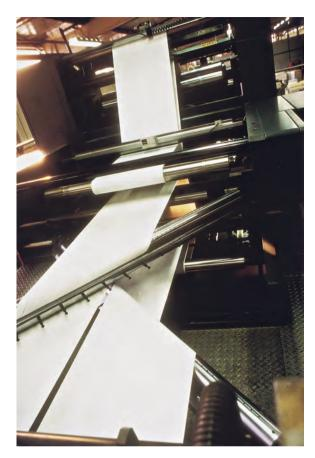
Fig. 2.1-100 Turner bars for turning the web, changing web travel direction and position (Heidelberg)
