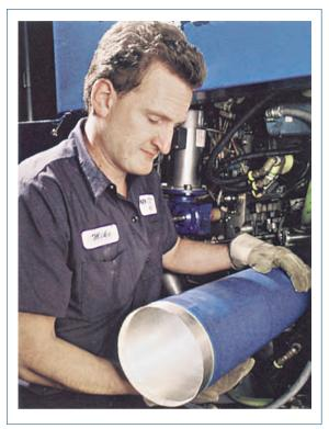
Fig. 2.1-104 Blanket cylinder sleeve (M-3000, Heidelberg)
