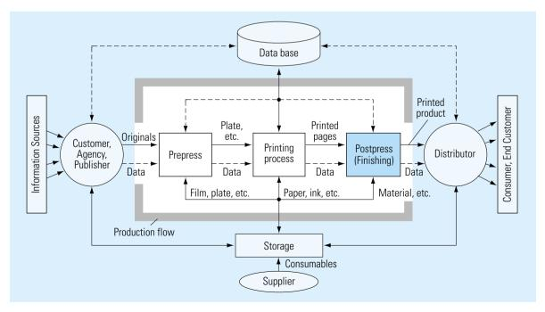
Fig. 7.1-1 Production flow of materials and data for the creation of printed products
