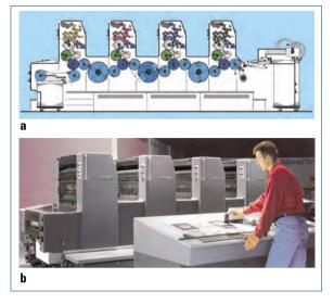
Four-color sheet-fed offset press with a central control console and measuring and control technology.
