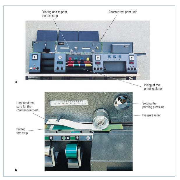
**Fig. 1.7-16** Test printing system. **a** Structure of the system;
