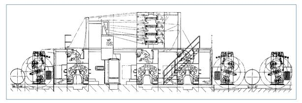
Fig. 2.1-197 Single-level design of a web printing system with Y-type printing units for newspaper printing (IFRA/MAN Roland)
