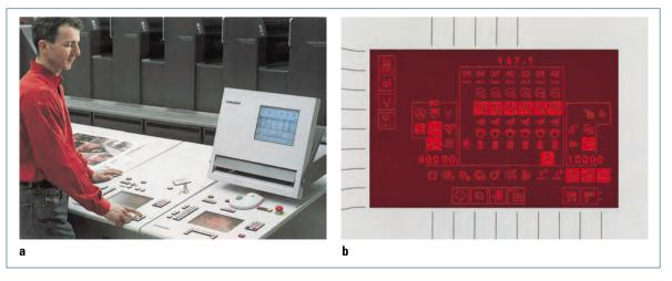
Fig. 2.1-168 Control console for the remote control of a sheet-fed offset press.
