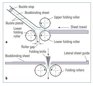
Fig. 7.2-22 Folding principles in sheet folding machines. a Buckle fold principle; b Knife fold principle
