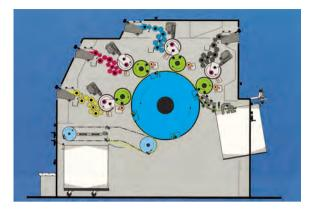
**Fig. 2.1-217** Computer to press/direct imaging printing system (ΩM DI 46-4, Heidelberg)
