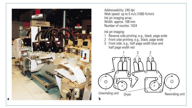
Fig. 1.3-32 High-speed ink jet printing system (System 6240/Color Runnar, Scitex Digital Printing/Matti Technology)
