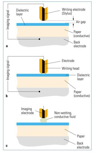
Fig. 5.7-1 Creating a latent image in electrography. a Writing electrode (stylus) is not in contact with the substrate; b Writing head is in contact with the substrate; • Writing electrode is in contact with the dielectric layer of the
