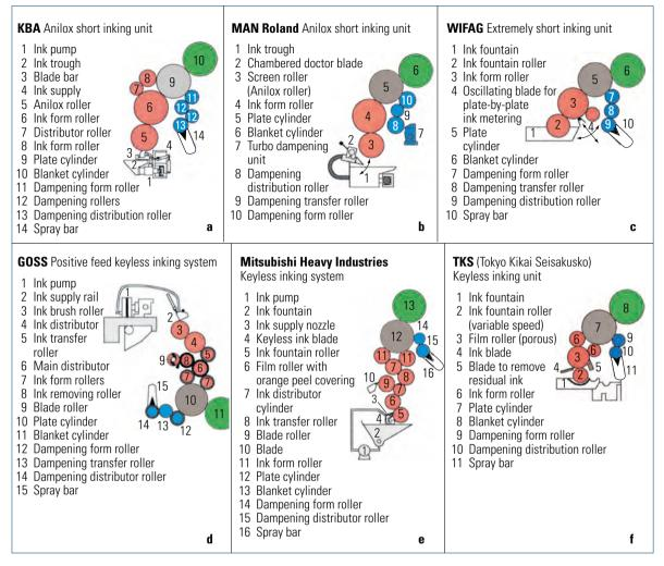
Fig. 2.1-122 Examples of keyless inking units (KBA)
