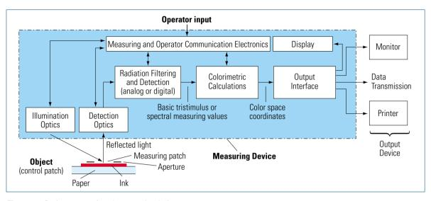
Fig. 1.4-48 Basic structure of a color-measuring device
