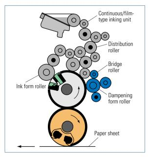
**Fig. 13.1-44** Model inking unit for simulation with INKTEAM [13.1-14]
