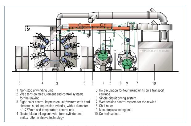
Fig. 1.6-22 Eight-color central impression cylinder flexographic printing press, reel to reel operation (W&H)
