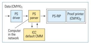
Color transformation with PostScript parser technology (PS parser software module within the computer) for adapting the proof printer (case 5)
