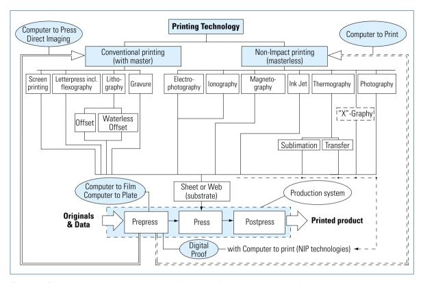
Fig. 4.5-19 Printing processes, computer to ... technologies, and workflow for the production of print media
