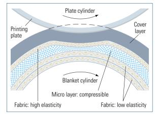
Fig. 2.1-46 Structure of a compressible blanket (ContiTech)
