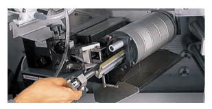
Fig. 2.5-28 Rotary screen printing module for label printing (Gallus/ Heidelberg)
