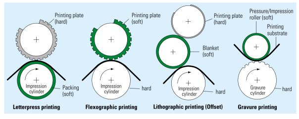
Fig. 1.6-2 Printing unit cylinders with radial flexible layers
