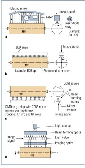
Design variants of multibeam systems for optical imaging with electrophotography.
