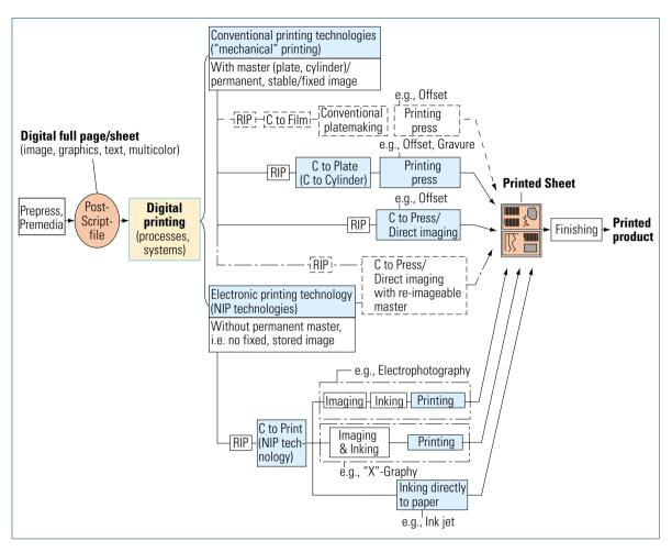
Fig. 6.1-2 Digital printing: technologies, components, and systems
