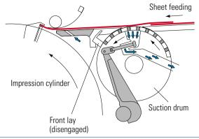
Fig. 2.1-36 Suction drum system (KBA)
