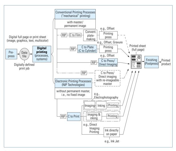
Fig. 4.5-18 Digital printing technologies, components, and systems
