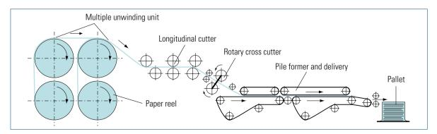
Fig. 7.2-11 Rotary cross cutter (cutting 4 webs)
