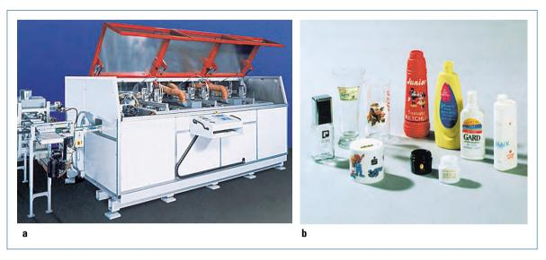
Fig. 2.4-16 Multicolor automatic screen printing machine for printing on bottles, glasses, etc. a Automatic machine (EC/4F); b Samples of printed products (ISIMAT)
