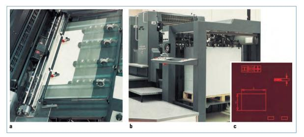
Fig. 2.1-160 Automated sheet size adjustment at the feeder of a sheet-fed offset press.
