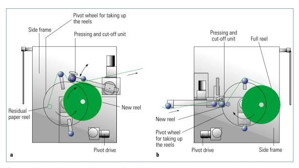
Fig. 2.2-39 Non-stop winders for unwinding and rewinding with fully automated reel change on gravure packaging printing presses. a Unwinding unit;
