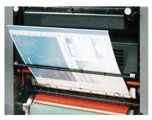
Fig. 2.1-43 Automatic plate loading (Speedmaster SM 52, Heidelberg)
