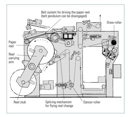
Gravure printing reel stand for flying reel change with one drive belt located at the bottom as support for the paper reel (KBA)
