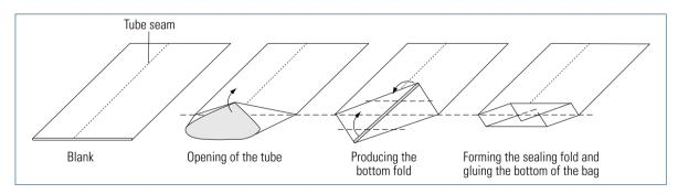
Fig. 7.3-36 Forming a cross bottom from a paper tube
