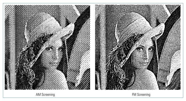
Fig. 1.4-38 Comparison of amplitude-modulated (AM) screening with frequency-modulated (FM) screening (AccuTone, R. R. Donnelley)
