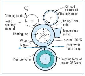
Fig. 5.2-17 Fixing unit (Océ; [5.2-3])
