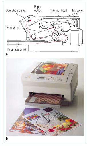
**Fig. 5.6-13** Multicolor thermography printing systems. **a** Equipment diagram for thermal transfer printing system (Mitsubishi Electronic); resolution 300 dpi, (256 addressable gray values), Format A3+, 3 minutes per A3 print;
