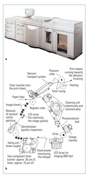
Computer to print system for single-color printing and in-line production of print media (electrophotography, LED imaging on photoconductor belt, 110 A4 pages per minute).
