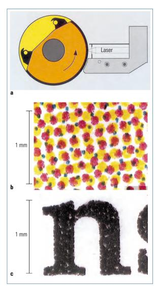
Fig. 4.4-7 Imaging the plate by means of laser ablation. a Imaging method;
