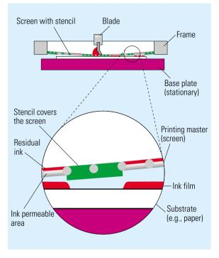
Fig. 1.3-22 Screen printing (schematic diagram)
