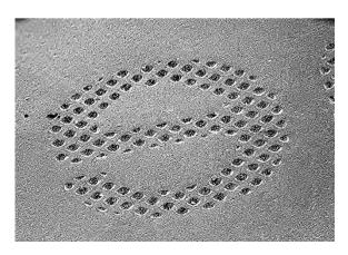
Fig. 3.1-53 Microphoto of a gravure cylinder
