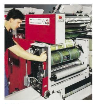
Fig. 2.5-19 Exchanging the slide-in printing unit for the variable-format (e.g., cut-off range: 432 mm to 711 mm) offset print (A68, Müller-Martini)
