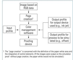
Fig. 3.2-68 Making a proof including the linking up of output profiles
