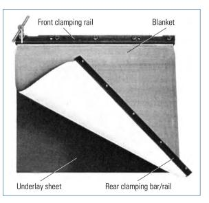
Fig. 2.1-47 Fixing the blanket (pre-railed blanket)
