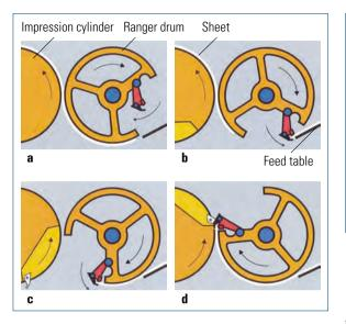
Fig. 2.1-34 Ranger drum, sequence of functions.
