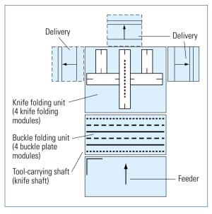
Fig. 7.2-36 Configuration of a combined folding machine
