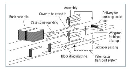
Fig. 7.2.-94 Casing-in machine (Kolbus)
