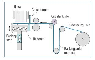
Fig. 7.2-68 Crossways lining station (back-stripping machine) [7.2-4]
