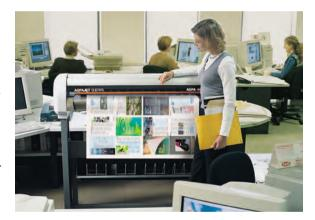
Fig. 3.2-74 Imposition color proof with large-format ink jet printer (Sherpa, AGFA)
