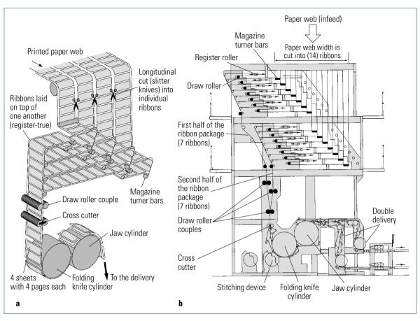
**Fig. 2.2-18** Cutting and folding in rotogravure/gravure printing.
