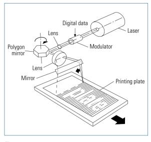
Fig. 4.3-7 Design principle of a flat-bed plate imagesetter: The printing plate is held on a flat table
