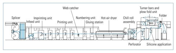
Fig. 1.6-9 Print line of a web-fed offset printing press with the individual units (IFRA/KBA)
