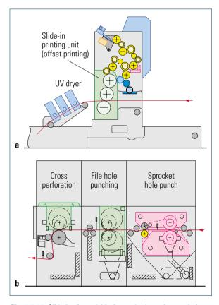
Fig. 2.5-20 Slide-ins for variable-format business forms printing. a Offset printing unit;
