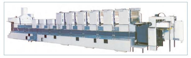
Lithrone 40, 6-color press, two coating units, unit for intermediate drying, hot-air extraction in the delivery; sheet size 720 mm × 1030 mm, printing speed 15000 impressions/hour (Komori)
