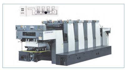
Shinohara 66 IVP, 4-color press with sheet reversal. Printing units 1 and 2 are connected by a double-size transfer cylinder, as are printing units 3 and 4. Sheet reversal with a 3-drum system after the second printing unit; sheet size 483 mm  $\times$  660 mm, printing speed 13000 impressions/hour (Shinohara)
