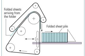
Fig. 7.2-35 Upright sheet delivery on a folding machine
