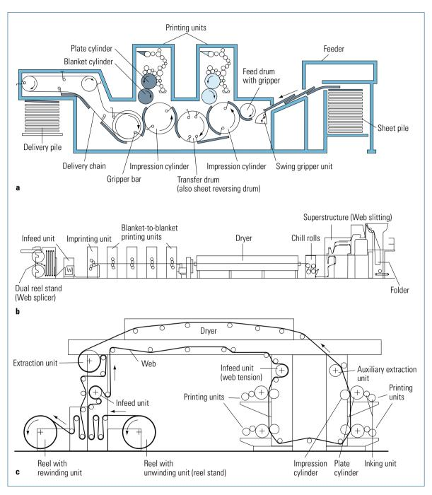
Fig. 1.6-4 Basic configuration of rotary presses.
