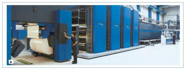
**a** Commercial web offset printing system (48 pages, double-sized cylinders, 50000 revs./hour, max. 100000 copies/hour, web speed 15 m/s) with zero-speed web splicer in horizontal design (M-4000, Heidelberg);
