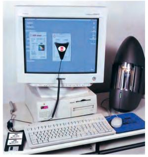
Fig. 3.2-67 Monitor color measuring system for the calibration of color screens (Vipview, FAG)
