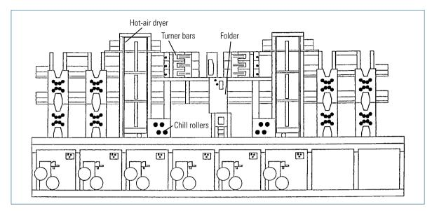
Fig. 2.1-202 Example of a web printing system with vertically configured hot-air dryers (IFRA/MAN Roland)
