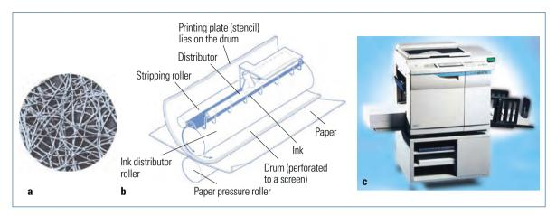
Fig. 2.4-20 Stencil/Screen printer for office applications.
