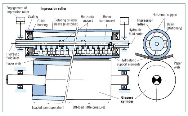
The principle of the deflection-compensated impression roller. A number of support elements inside the roller compensate the deflection of the gravure cylinder and ensure that the contact pressure remains practically constant along the entire web width (of the paper). A hydrostatic bearing is located between the immovable support elements and the rotating sleeve (NIPCO, Voith-Sulzer)
