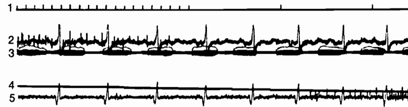
Figure 6.2. The electrical activity of several muscles of the chest during speech. The traces were recorded on an oscilloscope during the repetition of the syllable [mā]; (1) time marker, seconds; (2) decreasing electrical activity of the external intercostals; (3) acoustic signal recorded by microphone; (4) volume of air in the lungs gradually decreasing; (5) increasing activity of the internal intercostals. (After Draper, Ladefoged and Whitteridge, 1960.)
