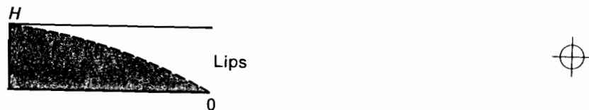
Figure 4.9. A uniform tube open at one end, showing a pressure waveform at the first formant frequency.
