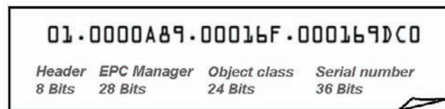
Figure 5. The electronic product code (Source: RFID Gazette, 2005)
