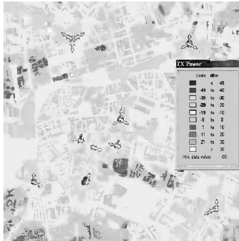
FIGURE 74.10 The required transmit power for the speech service.
