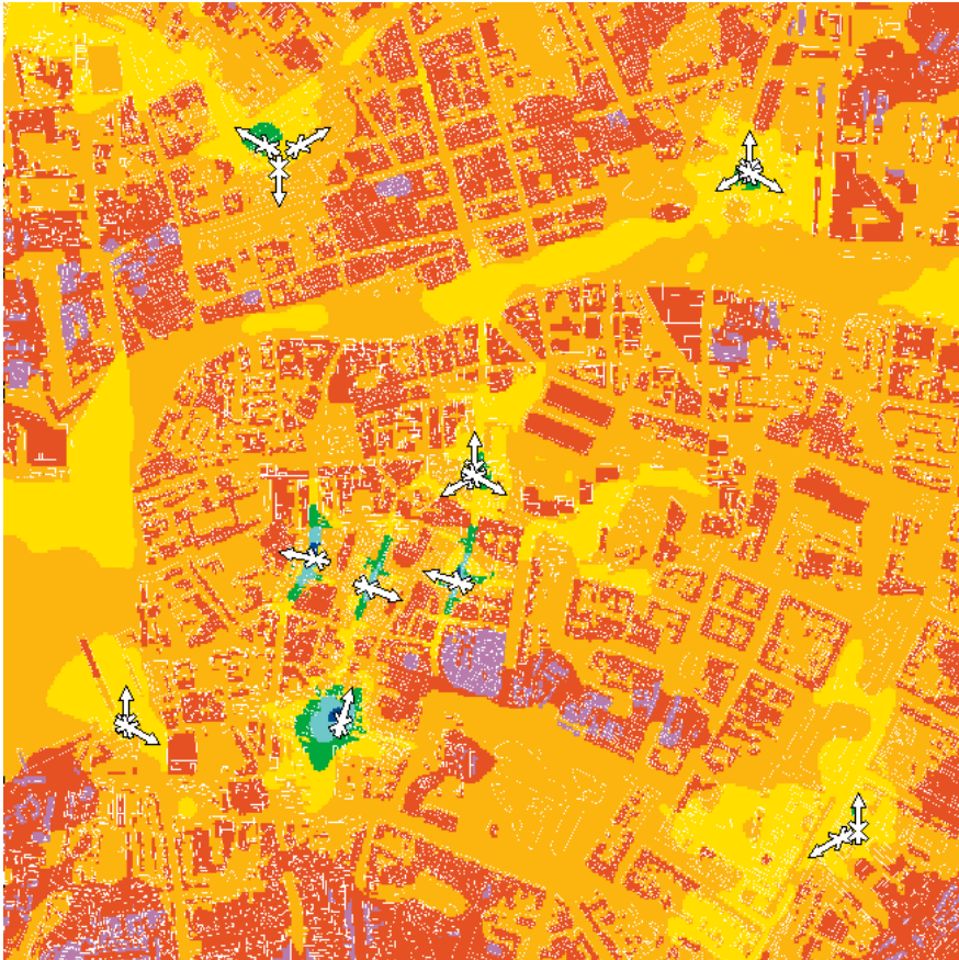
FIGURE 74.15 Required MS transmit power for the 384 kb/s high rate service. Original traffic levels shown in Figure 74.9 apply.
