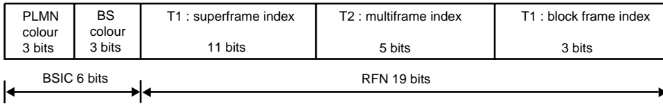
FIGURE 80.7 Synchronization channel (SCH) message format, ©ETT [4].
