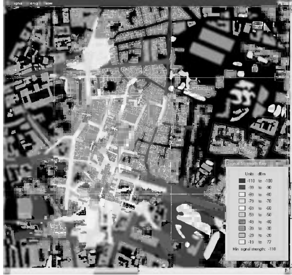
FIGURE 74.5 Cluster of microcells in a city centre. The map gridsize is 500 meters.
