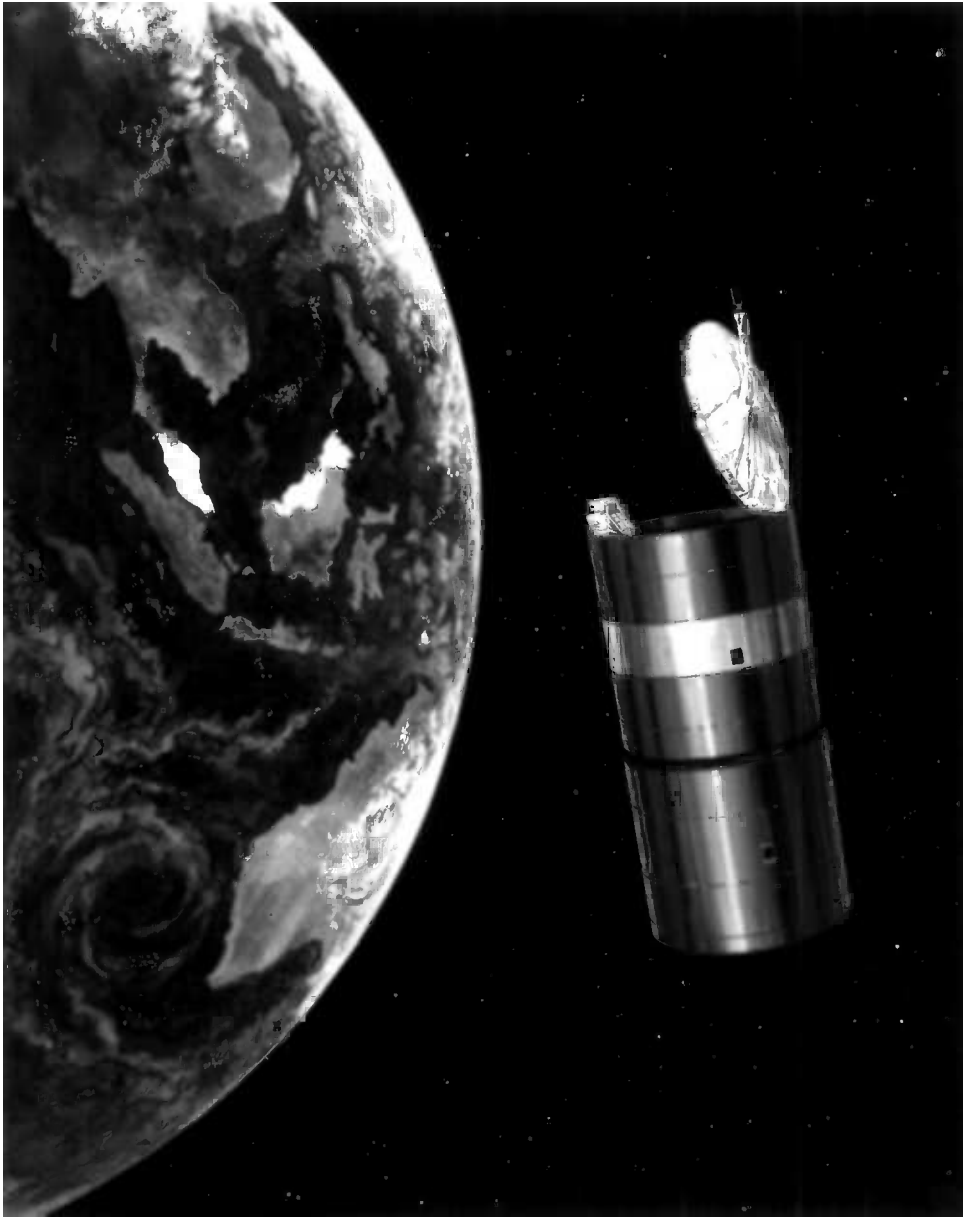
FIGURE 56.6 Measat, first launched in 1996, is a small satellite of the Hughes HS-376 class. With 1100 W of payload power, it provides both low-power C-band and medium-power Ku-band transponders to Malaysia and surrounding countries in the Asia–Pacific region. (Photograph courtesy of Hughes Space and Communications Company.)
