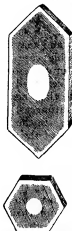
FIG. 103.—Conductivity coefficients of expansion; the one measured in the direction of the principal axis may be either greater or less than that measured in directions perpendicular to this axis. A sphere cut from a uniaxial crystal at one temperature will be a spheroid at another temperature. In biaxial crystals there are different coefficients of expansion along three rectangular axes, and a sphere at one temperature will be an ellipsoid at another. A result of this is that for all crystals, except those belonging to the cubic system, the angles between the faces will vary, though only slightly, with changes of temperature. E. Mitscherlich found that the rhombohedral angle of calcite decreases 8' 37'' as the crystal is raised in temperature from 0^\circ to 100^\circ C.
