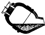
FIG. 17.—Bessemer Converter, turned down in position to receive and discharge the molten metal.
