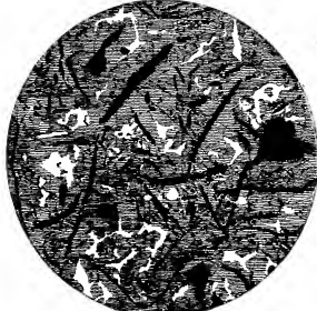
FIG. 27.—Graphite in Grey Cast Iron.
