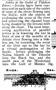
FIG. 4.—Mississippi South Pass Outlet Jetty.
