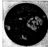
FIG. 9.—PORPHYRITIC AND FLUIDAL RHYOLITE, HUNGARY (×12).
