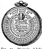
FIG. 71.—Wynne's "Infallible" Exposure Meter.
