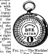
FIG. 70.—The Watkins's "Bee" Meter.
