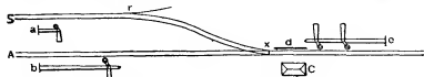
FIG. 5.—Interlocked signals (American practice, signals at right track, and arms at right of post).
