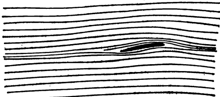
FIG. 17a.—Flow past wing 6°. Below critical angle.
