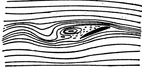
FIG. 17b.—Flow past wing. 20°. Below critical angle.
