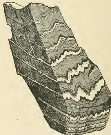
Fig. 54.—Sketch (by the late Mr Du Noyer) of a block of variegated slate from Devil's Glen, county Wicklow. The crumpled bands mark the bedding, and the fine perpendicular striae in front are the cleavage planes; the fine lines on the darkened side merely represent shadow, and must not be taken for planes of division in the rock. It will be observed that the cleavage planes do not pass through the white hands.
