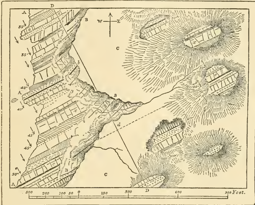
FIG. 18.—Geological map of a portion of a rocky coast-line, and the country inland. (J. B. Jukes.)
