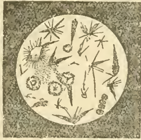
FIG. 3.—Microscopic Structure of Pitchstone. A glassy base, with numerous feathered and needle-shaped micro-lites, and a sanidine crystal.
