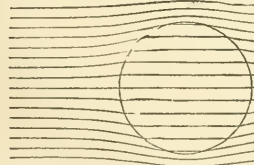
FIG. 33.—Lines of Force for a Diamagnetic Sphere.
