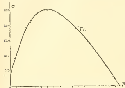
FIG. 35.—Curve \mu = \mathfrak{H} for Iron.
