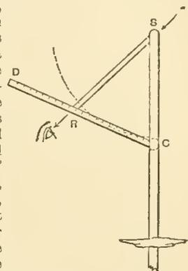
FIG. 4.—ST is the standard; SR the radius bar and pointer, with vanes and pinnles at the side; CD is a scale of chords which is lifted up to touch the pointer and indicate the angle from 90° near C to zero near D. By the size of the observer in the drawing the standard ST was 10 or 12 feet in length.
