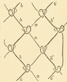
*Bobbin Net.* which is the foundation of machine-made lace, is made by the intertwisting—not knotting—of contiguous threads (see LACE, vol. xiv. p. 185).
