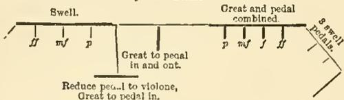
The swell pedals control two sides of the swell box and the orchestral oboe. The vox humana is in a box which is always shut. These swell pedals are on a new system, which admits of fixing them at any point, so that the tone can be determined to any strength.
