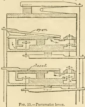
FIG. 13.—Pneumatic lever.
