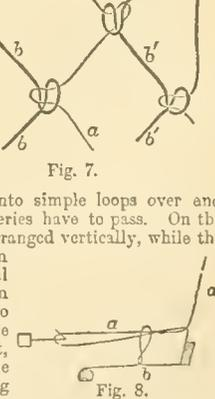
Fig. 8. Diagram of the machine mechanism for forming a mesh, showing threads 'a' and 'b' and the resulting loop.
